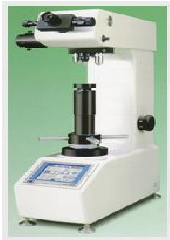
Figure 3.6: Future Tech Vickers Hardness Tester FV-700
