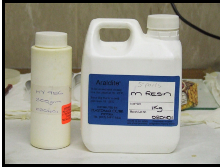
Figure 3.10a. Araldite M Resin and HY956 hardener (PLASTOMAX CC/BK). The resin based material was used for the embedding. The resin was mixed with a hardener in a ratio of five to one according to weight.
