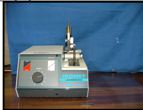
Figure 3.10d. The ISOMET (BUEHLER, Germany) is a low speed, water cooled, diamond tipped saw.
