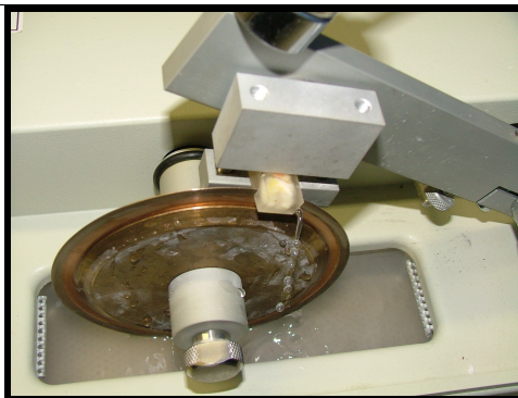
Figure 3.10e. The embedded tooth was sectioned at a speed setting of eight. [Diamond wafering blade, series 15HC diamond no. 11-4244 (BUEHLER®, USA)].
