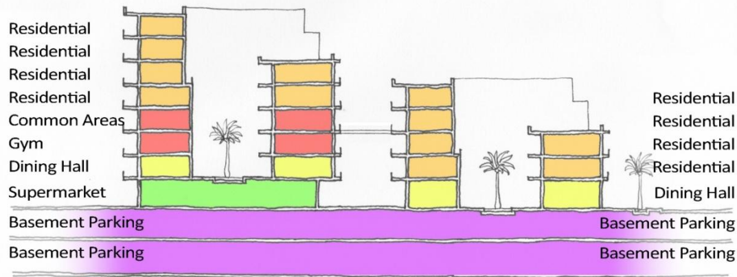
Figure 61: Section highlighting the location of functions within the buildings (Reference: author's own 2009)
