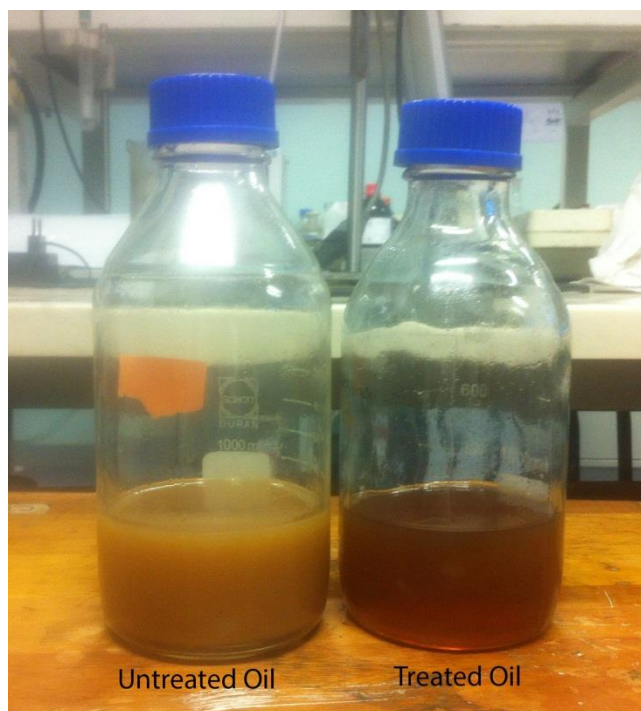
Figure 4.10: Waste cooking oil before and after treatment
