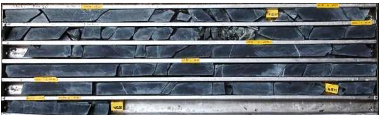
Figure 5.4: Komatiite in half core. Dark grey in colour with minimal textures evident.
