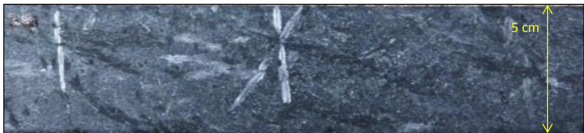
Figure 6.4: Pyroxene spinifex, showing randomly oriented needles. The shining X like needles is due to the reflection of the cleavage and the light.
