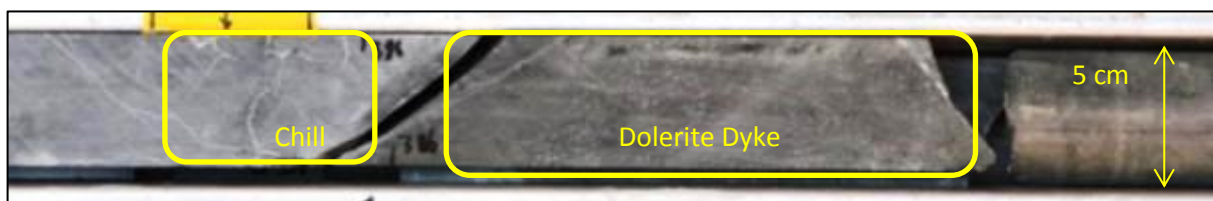
Figure 5.10: Dolerite dyke contact with underlying differentiated flow, clearly showing variole like features similar to the basalts.
