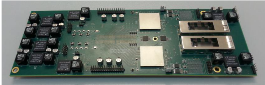
Figure 5.10: The Daughter-board for the upgrade system [2].
