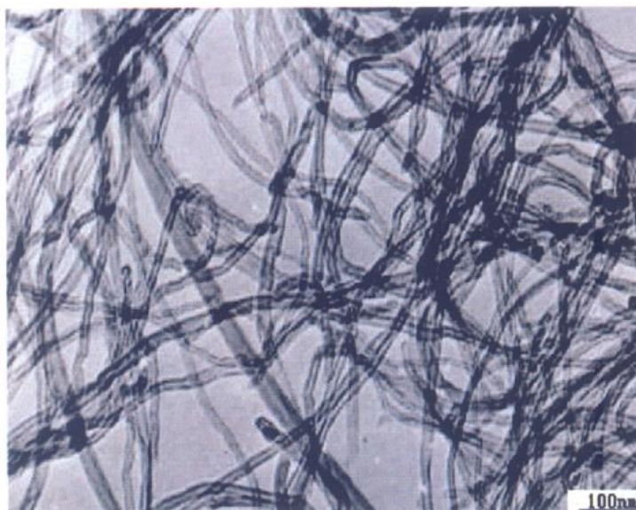
Figure 4.18: TEM showing the nanostructure image of MWNT
