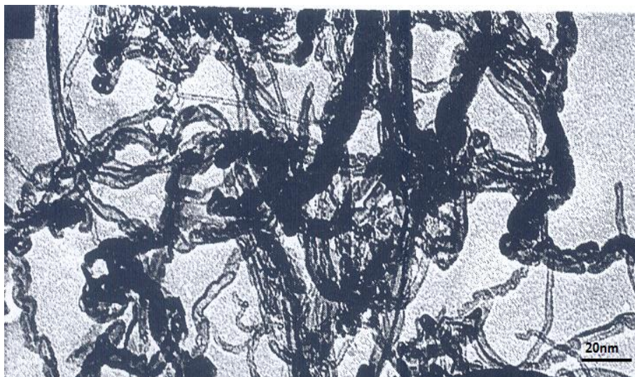
Figure 4.21: TEM showing the nanostructure image of the MWNT-PSI
