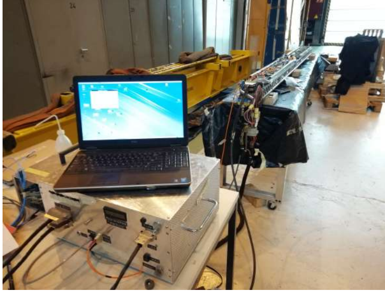
Figure 4.5: The MobiDICK system connected to the super-drawer during testing of the components
