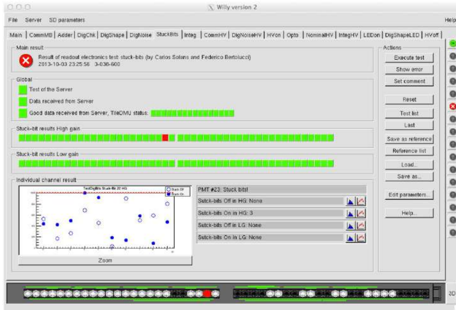
Figure 4.4: The Willy GUI showing the Stuck bits test [44]
