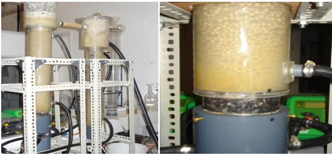
Figure 3.2 (A) Image of the AFGB column with CAC coated with bacterial flocs (biofilm) (B) shows the full bed granulated AFGB during fermentative biohydrogen production.
