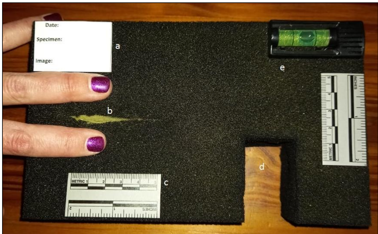
Figure 2.1: Foam block system utilized to photograph specimens. a: information tag; b: incision to accommodate articular/transverse process; c: scale bar; d: cutout to accommodate spinous process; e: spirit level.
