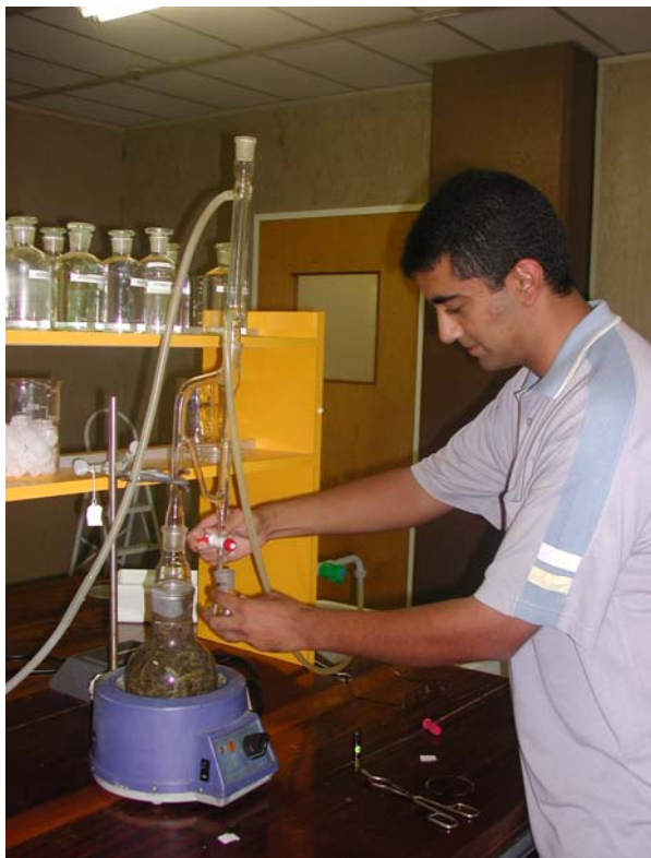
Figure 2.1 Isolation of essential oil by hydrodistillation of chopped air-dried plant material.
