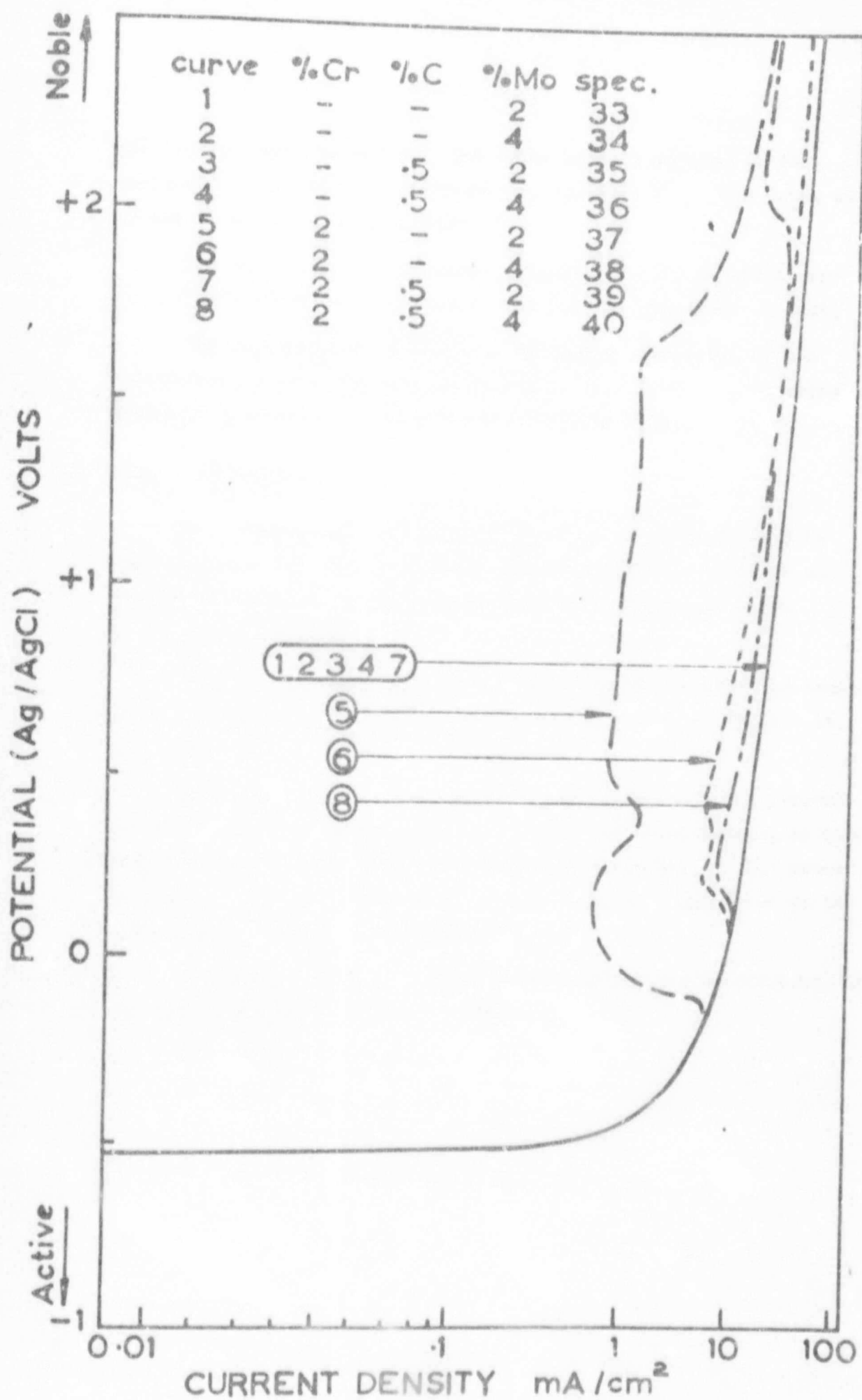
FIGURE 20: Polarization diagrammes showing influence of alloying elements on shape of curve. 12.5% Si alloys. 2.5% HCl.
