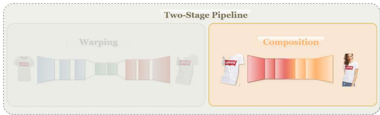
Figure 2.15: Composition represents the final stage in virtual try-on, where the warped clothing is composited onto the individual using a generative network.
