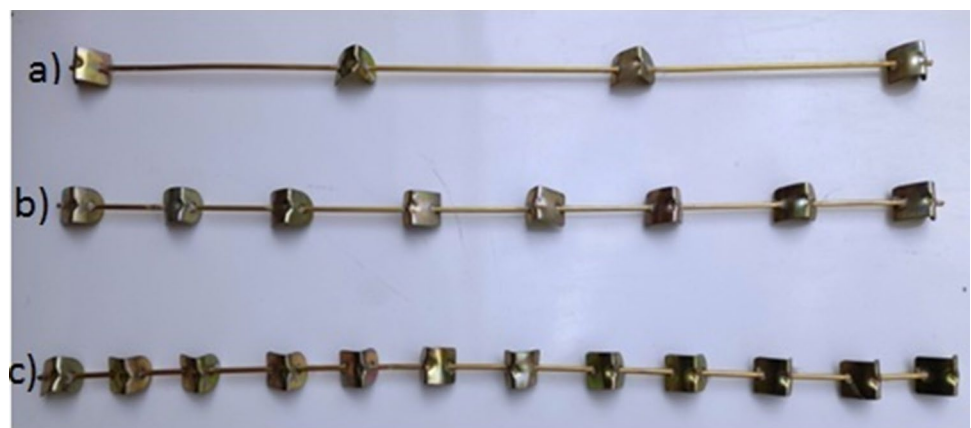
Fig. 1 Applied triangular baffles at 70^\circ and 40^\circ angles: a 4 baffles; b 8 baffles; c 12 baffles
