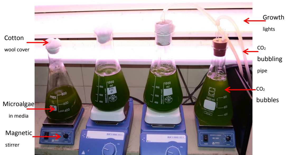
Figure 2.1: An illustration of algae growth set-up. Green microalga cells cultured in a modified Beijerinck medium, with periodical CO 2 bubbling
