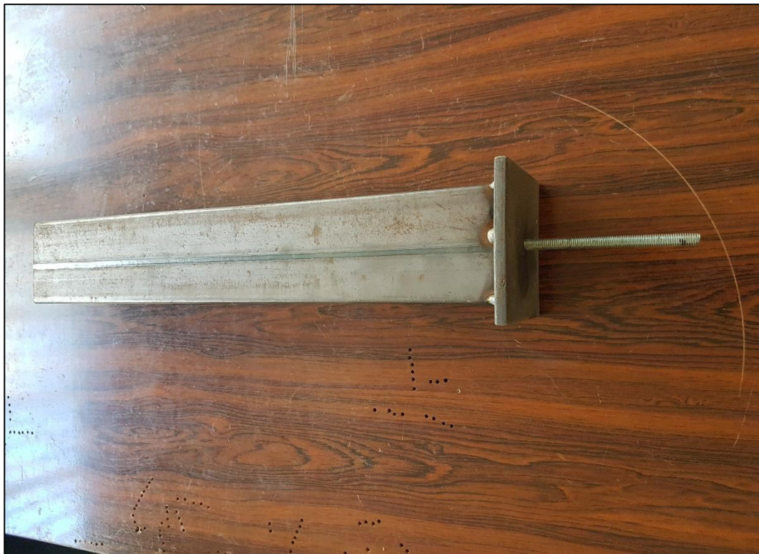
Figure C- 6: 100 mm square cylinder. (original hollow section steel)
