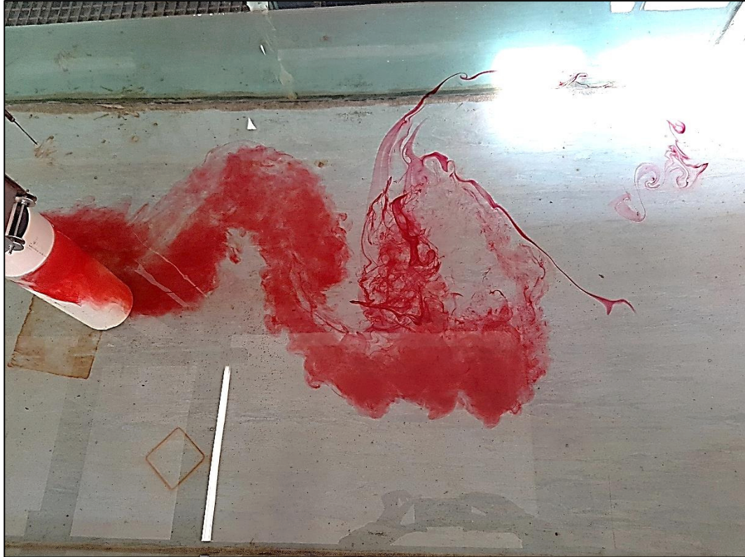
Figure 4-10: Photograph of von Kármán vortex street behind test cylinder
