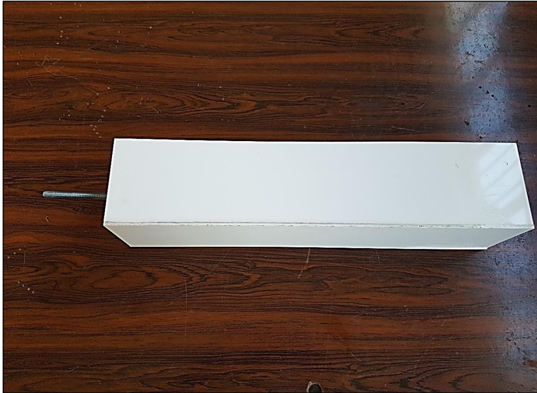
Figure C- 7: 100 mm square cylinder (Perspex box)
