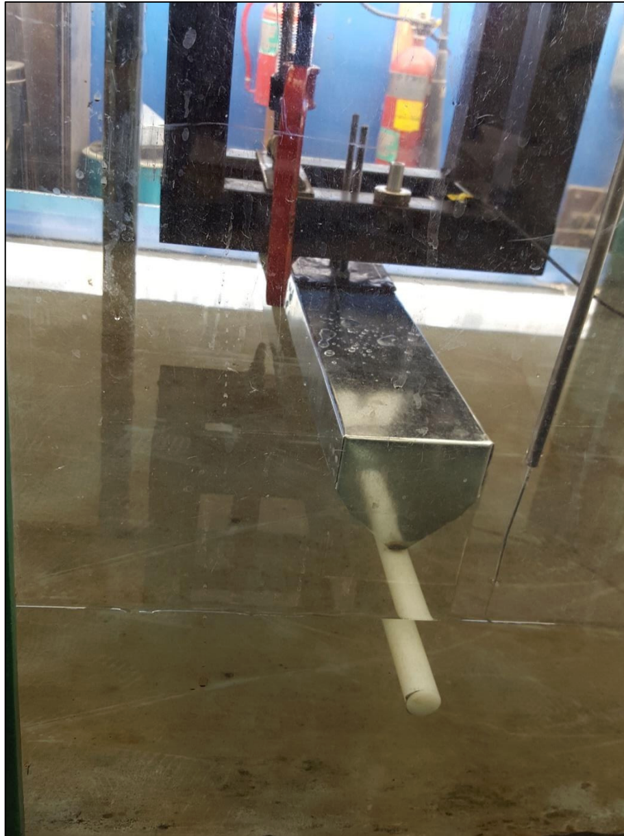
Figure B- 4: Photograph 2 of "infinitely' long cylinder apparatus for verification test
