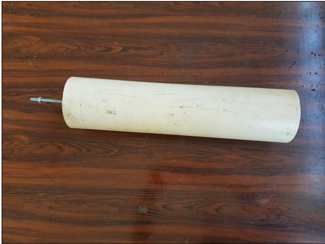
Figure C- 3: 110 mm diameter, 450 mm long circular cylinder
