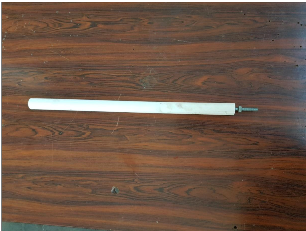
Figure C- 4: 25 mm diameter, 450 mm long circular cylinder
