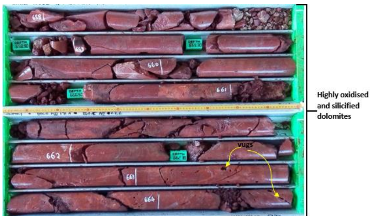
Figure 4-18: Photo showing the highly oxidised and silicified dolomites of the Chingola Dolomite Formation in borehole KN191A.
