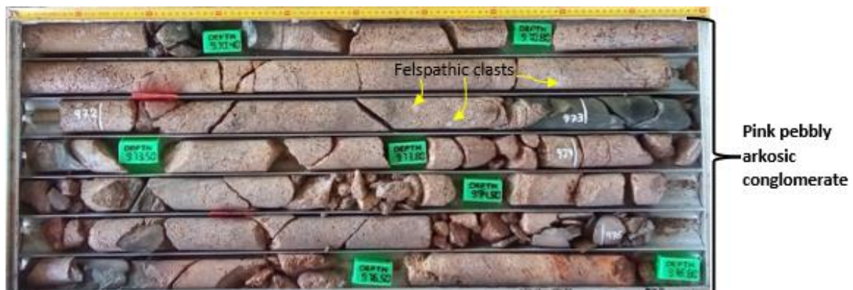
Figure 4-15: Photo showing the bedded pebbly arkosic conglomerate of the Konkola Member in borehole KN120.
