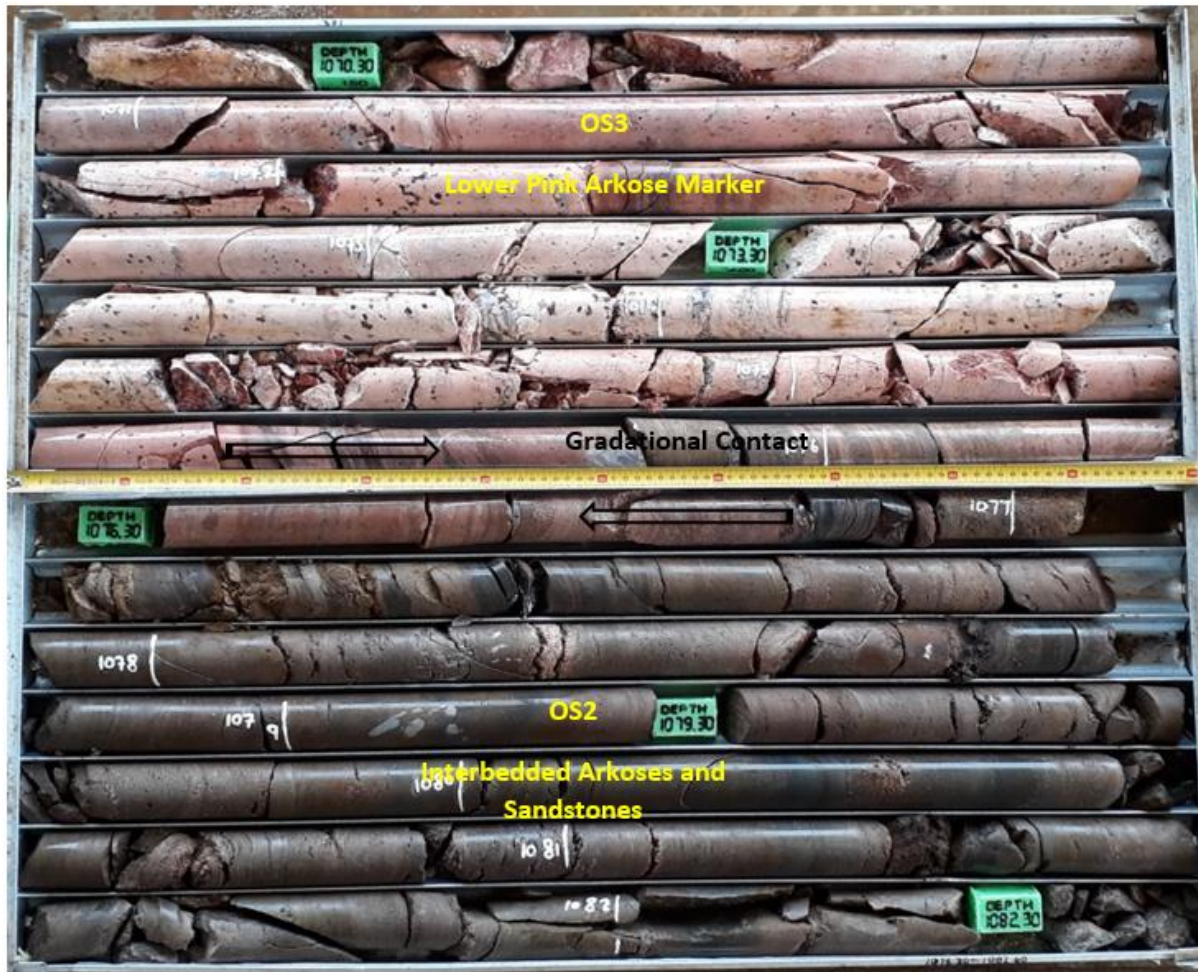
Figure 4-11: Photo showing OS2 Member (greyish interbedded arkose and sandstones) and OS3 Member (Lower Pink Arkose Marker) from borehole KN190.
