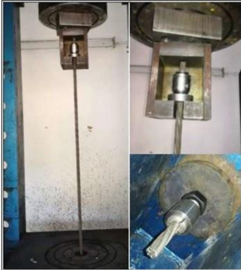
Figure 5-7: Photographs indicating laboratory UTS tests conducted on 4.5 m long 18 mm diameter cable steel samples at the Groundwork testing facility (Matitsela, 2018)
