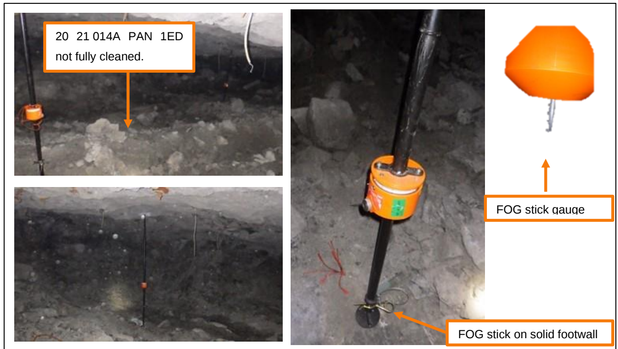
Figure 5-33: Photographs of FOG stick installation in 20 21 014A PAN 1ED Production output
