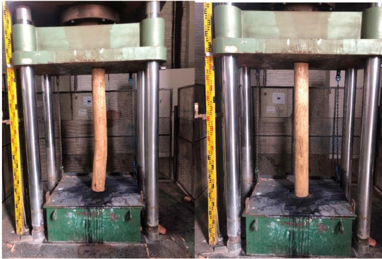
Figure 5-2: Laboratory compression tests conducted on 1.5 m long timber elongates.
