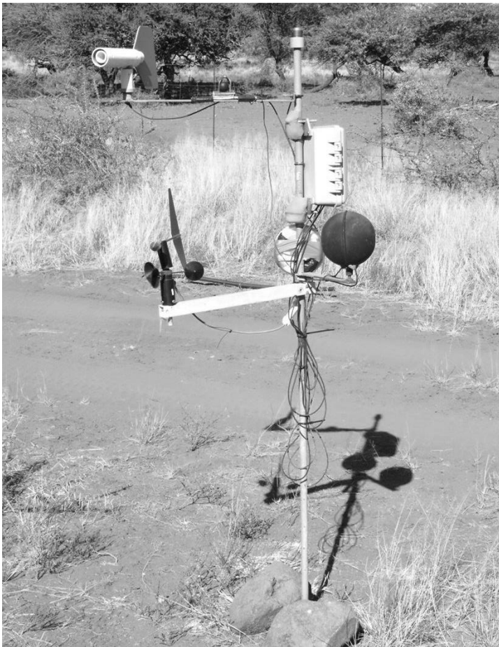
Figure 2.10 The weather station set up in an open area in Mokala National Park to measure dry bulb and black globe temperature, solar radiation, wind speed and direction, and relative humidity.
