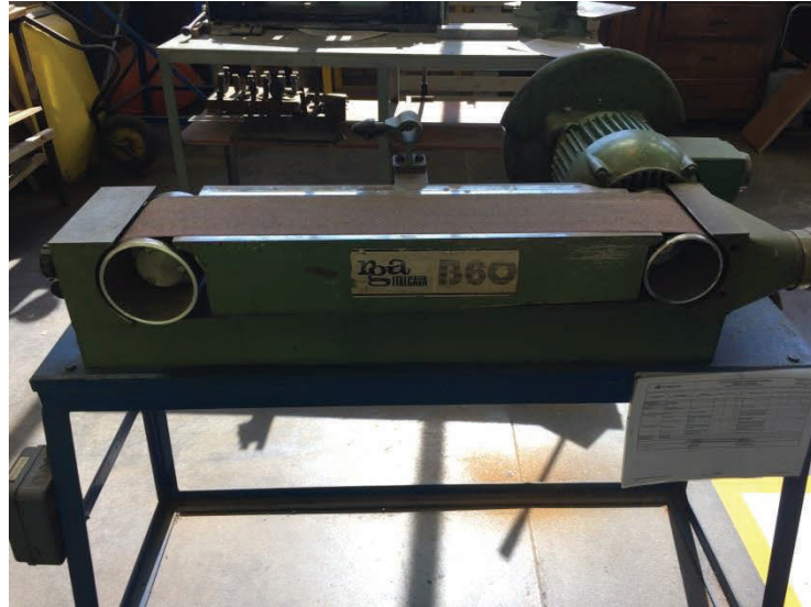
Figure 3-10: Belt sander used to remove the burr from the samples
