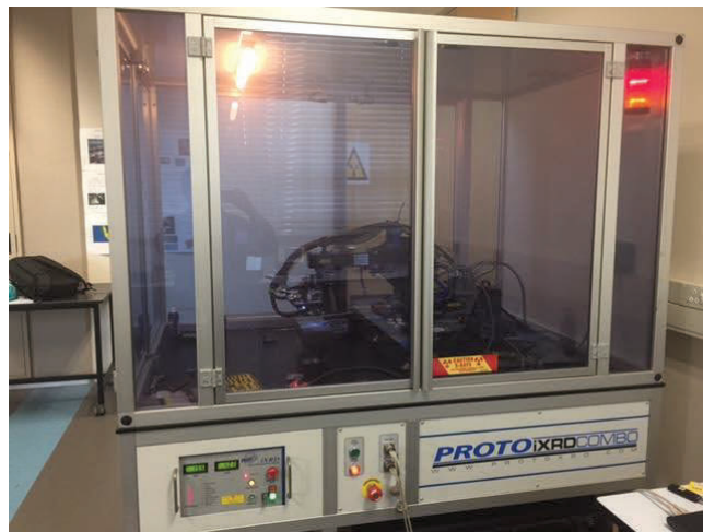
Figure 3-22: The ProtoiXRD COMBO used for measuring the residual stresses
