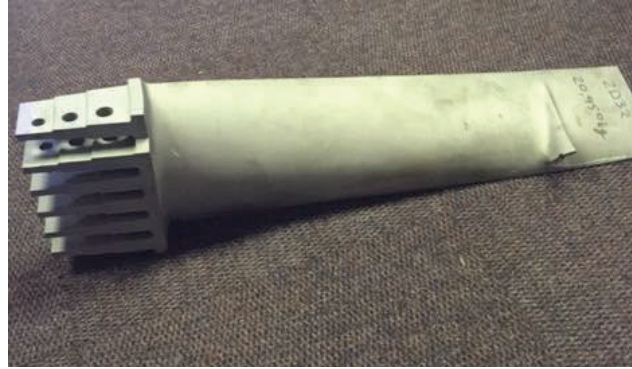
Figure 3-3. The original LP turbine blade before machining
