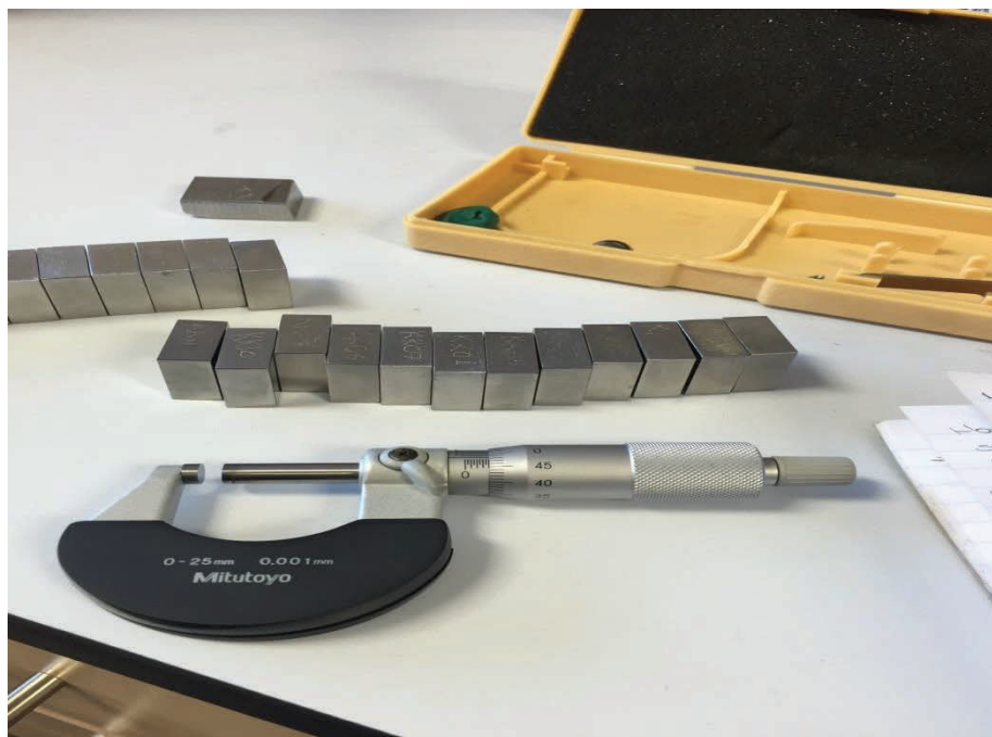
Figure 3-14: Micrometre used to confirm measured thickness of samples
