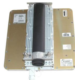
Fig. 17. Alvarion transceiver with massive heat sink fins.
