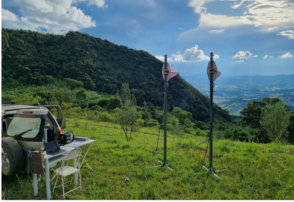
Fig. 16. Setup used for the 5G-RANGE field tests.
