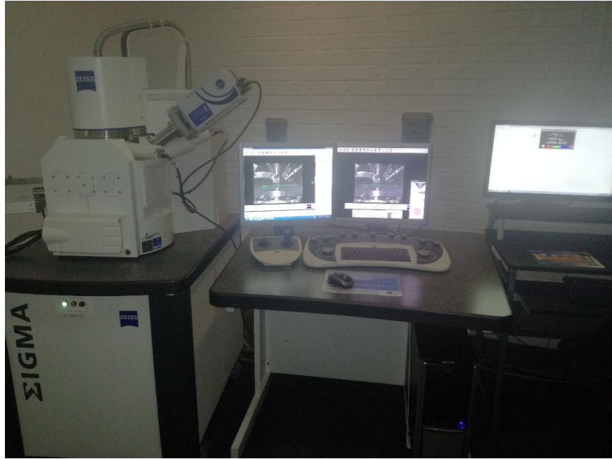
Figure 3.2: The scanning electron microscopy (SEM) used in the imaging and elemental composition determination of the deposited thin film.
