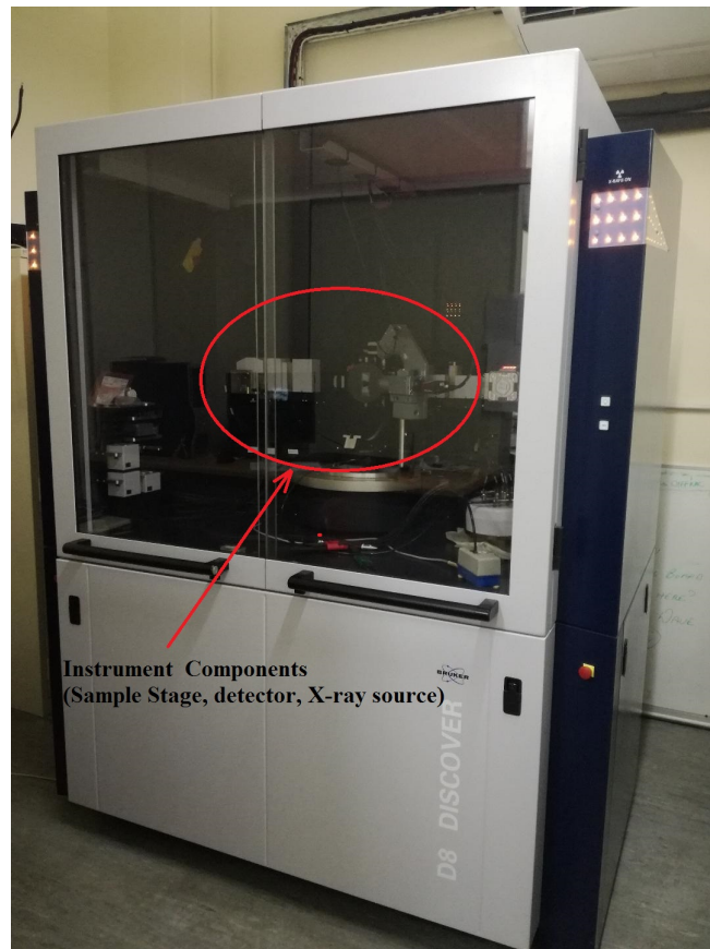
Figure 3.3: The AXS Bruker D8 Discover X-ray diffraction instrument used for GIXRD and XRR measurements.
