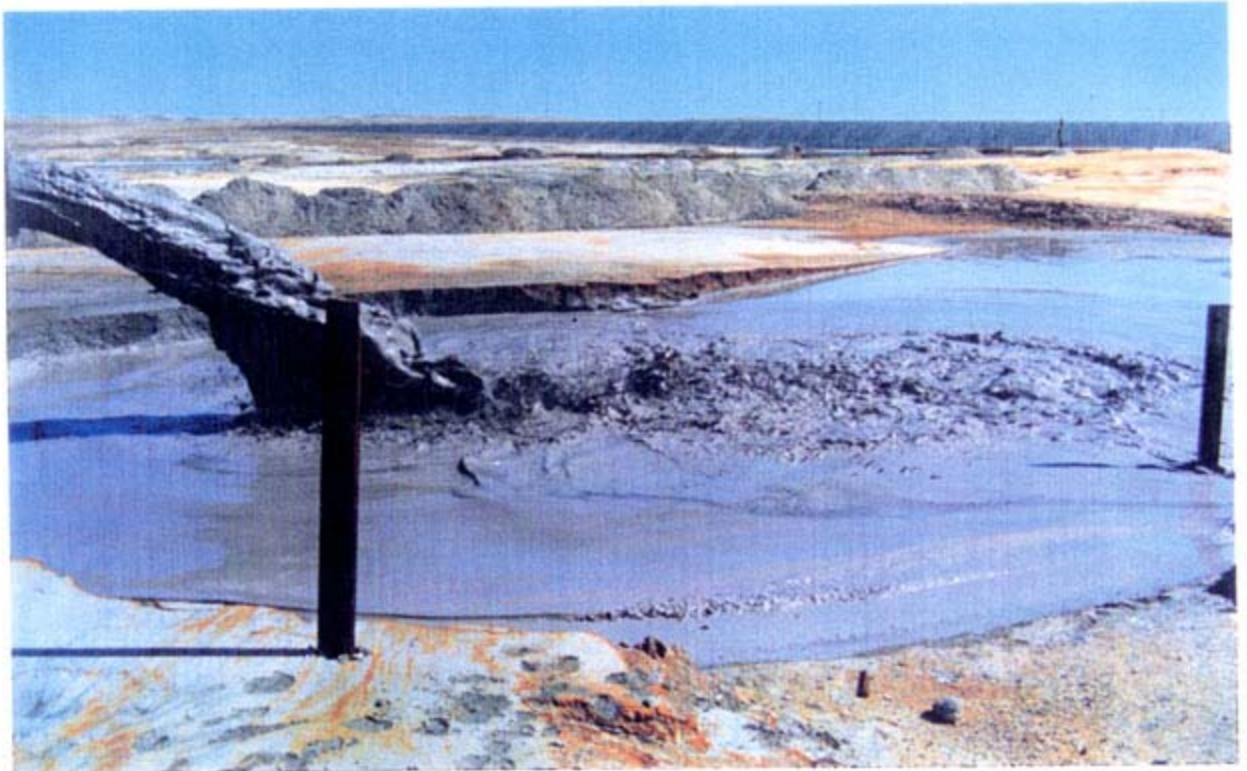
FIGURE 7.4 : PHOTOGRAPHS SHOWING THE DISCHARGE OF TAILINGS DURING THE TEST ON PADDOCK ST
