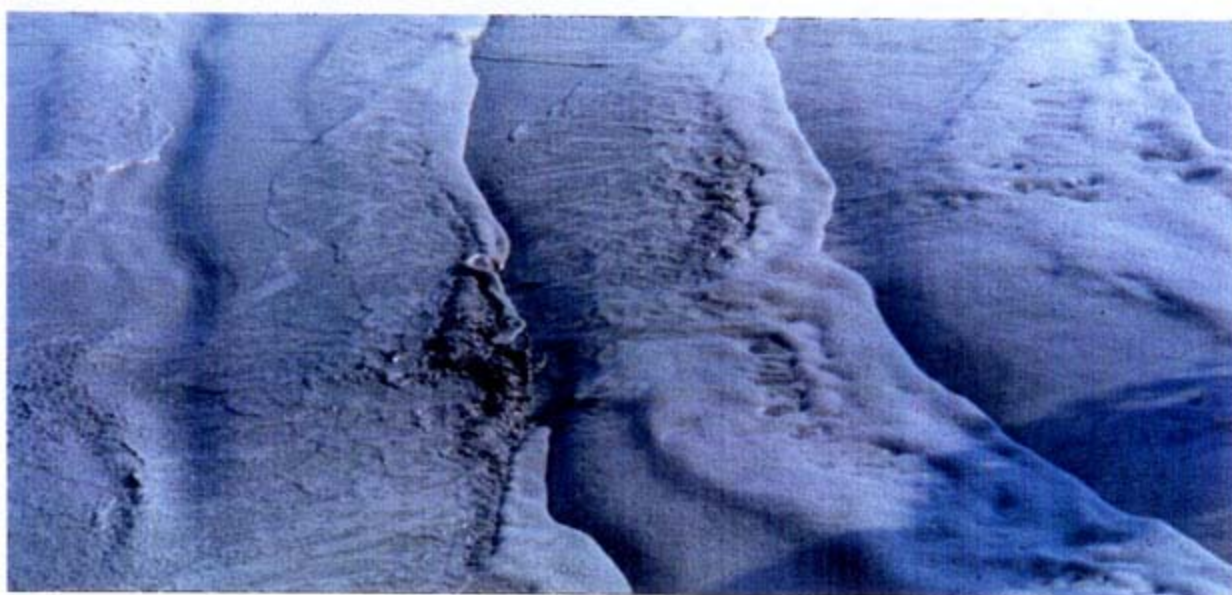
FIGURE 3.9 : PHOTOGRAPHS ILLUSTRATING THE UNSTEADY NATURE OF FLOW FROM A TAILINGS SLURRY DISCHARGE
