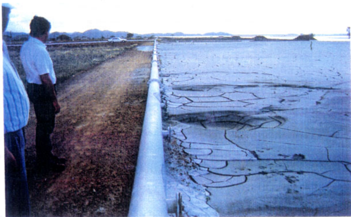
FIGURE 8.15 : PHOTOGRAPHS SHOWING TYPICAL DISCHARGE CONDITIONS DURING DEPOSITION TRIALS
