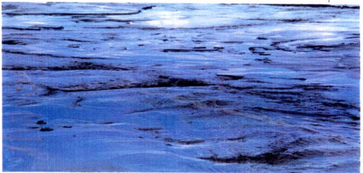
FIGURE 3.10 : PHOTOGRAPHS ILLUSTRATING THE UNSTEADY NATURE OF FLOW FROM A TAILINGS SLURRY DISCHARGE
