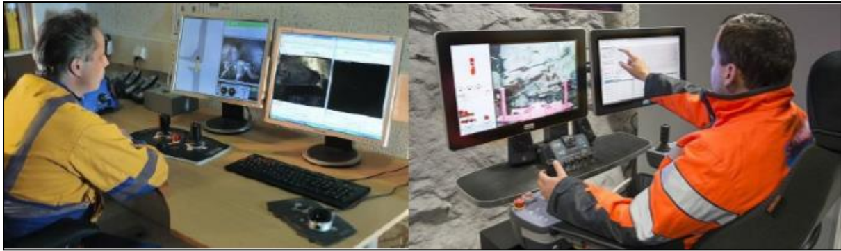
Figure 2-1: Control Room of an Automated Loading Operation (Marklund, 2017)
