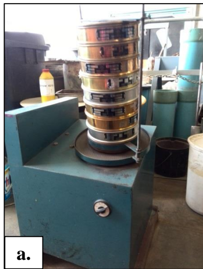
Figure 4.3: Sieve stack configuration (a) and hydrometer measurements setup (b)
