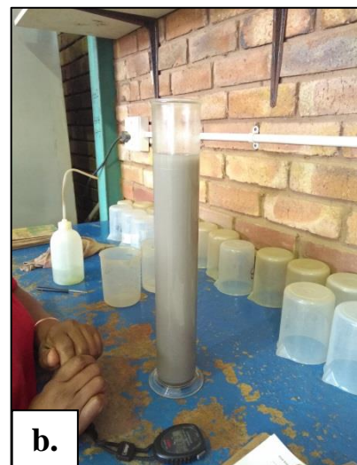
Figure 4.3: Sieve stack configuration (a) and hydrometer measurements setup (b)
