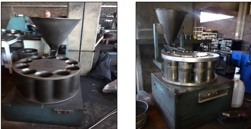
Figure 4.1: Two different size rotary splitters used for sampling (size reduction)
