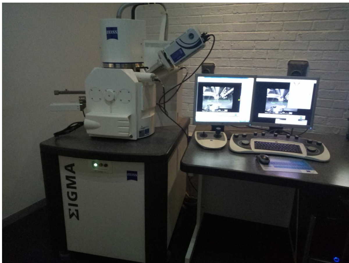
Figure 3.10 Image of Carl Zeiss Sigma Field Emission Scanning Electron Microscope equipped with an Oxford X-act EDS detector
