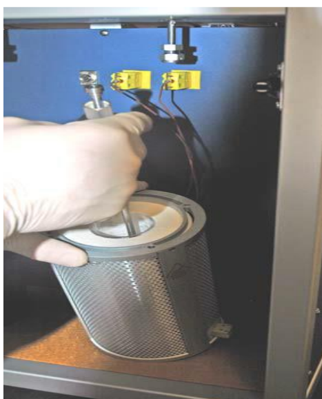
Figure 3.16 Connecting the furnace thermocouple cables to the Sample Compartment
