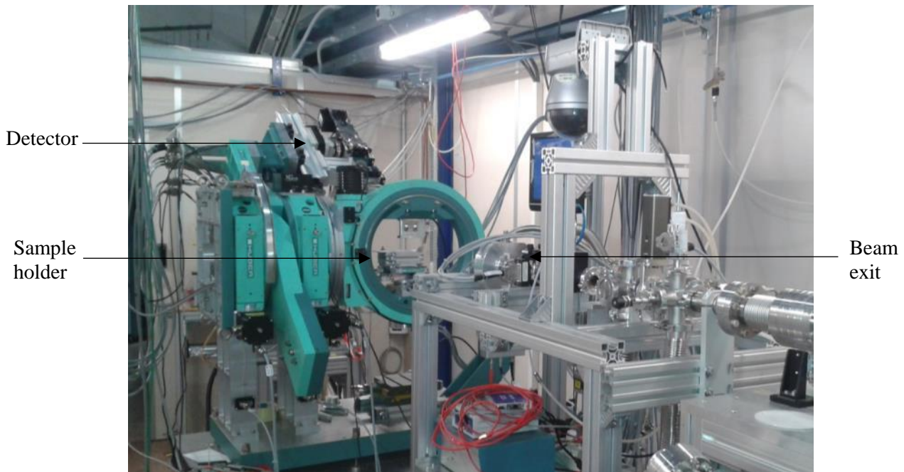
Figure 5.34 - Diffractometer of the Materials Characterisation by X-ray Work Station at Elettra
