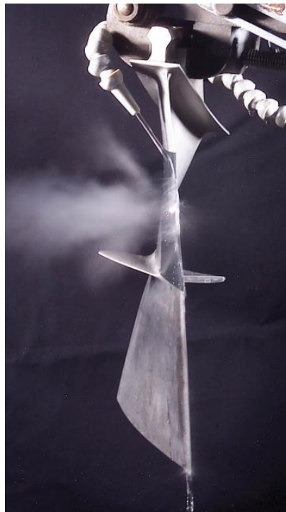
Figure 2.53 - Treatment of Compressor Blades Using Laser Shock Peening
