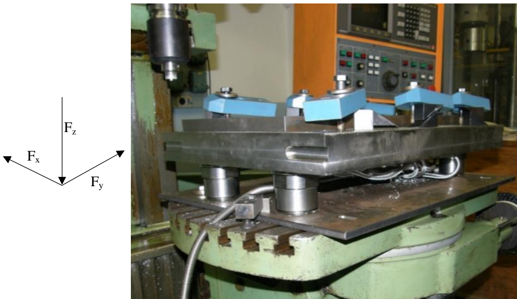
Figure 5.4 - Force Link Integrated into FSW Machine
