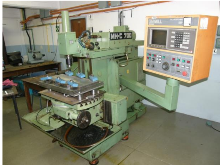
Figure 2.11 - Retrofitted Maho MH-C 700 CNC Friction Stir Welding Apparatus
