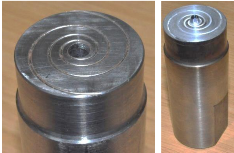
Figure 5.9 – Facetted Pin and Spiralled Shoulder Combination Friction Stir Welding Tool
