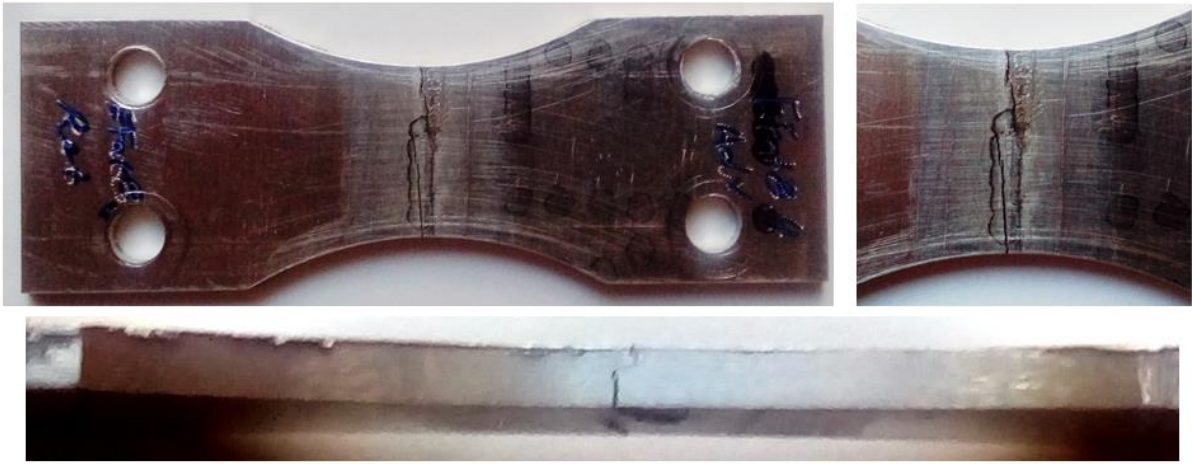
Figure 8.17 - Confirmation of Fracture of Friction Stir Welded Joints under Fatigue Loading
