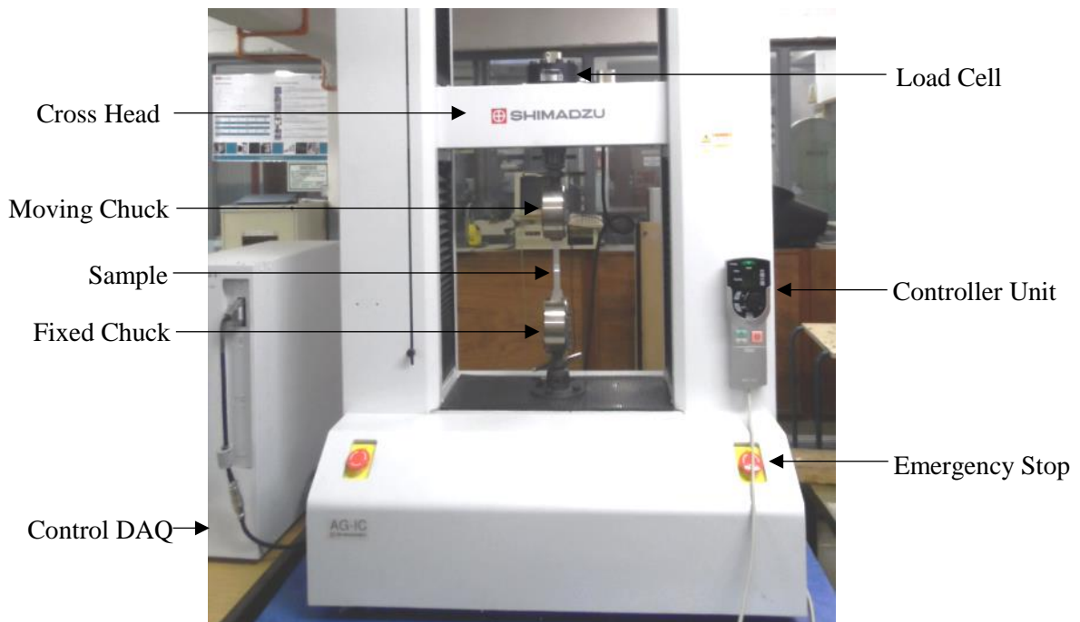
Figure 5.29 - Shimadzu AG-IC series Ag-20kN/50kNICD Electric Universal Tensile Tester
