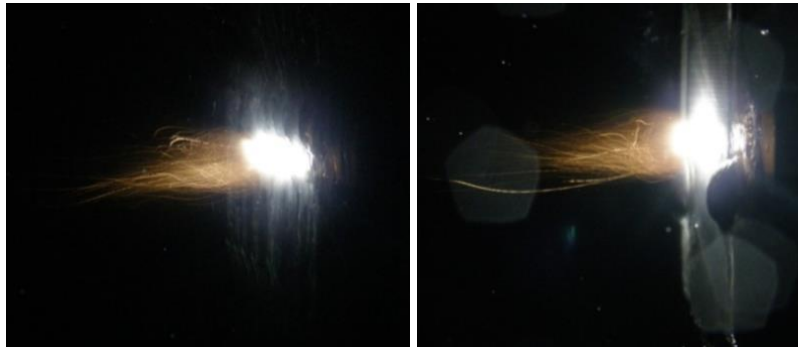
Figure 6.65 - Ablation of the Target Surface during Laser Shock Peening without a Protective Coating
