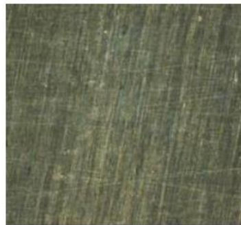
Figure 2.39 - Example of Imprint of Backing Plate on Friction Stir Welding Root Surface
