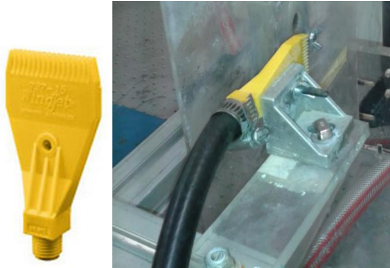
Figure 5.19- WindJet AA727 Nozzle and Integration into Laser Shock Peening Apparatus
