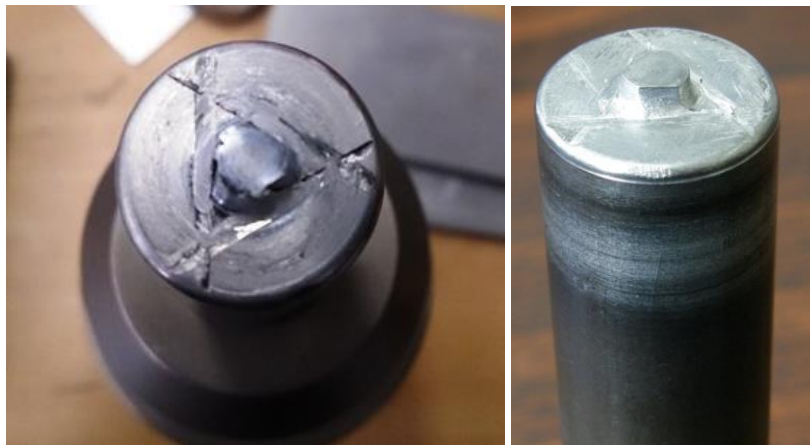
Figure 5.6 - Single Piece Friction Stir Welding Tool
