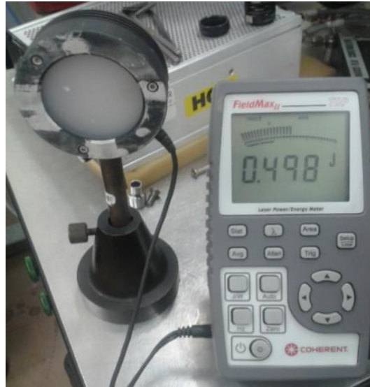
Figure 5.13 - Coherent Field Max II - Top Laser Power/Energy Meter
