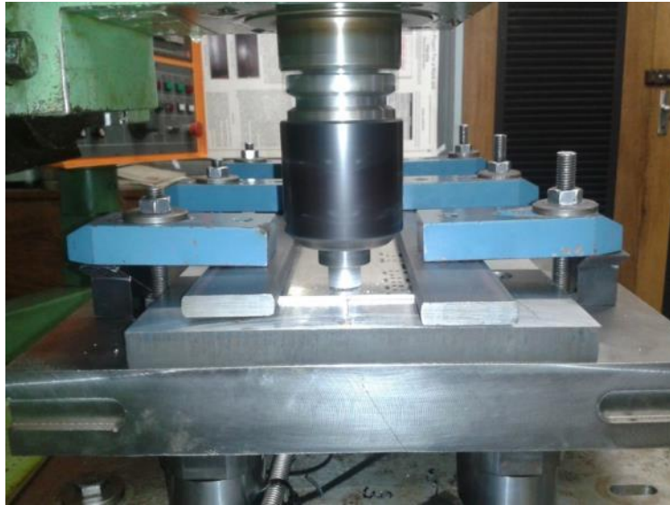
Figure 2.13 –Representation of the Backing bar Method
