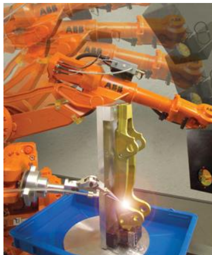
Figure 2.68 – Laser Shock Peening example of Laser Induced Breakdown
