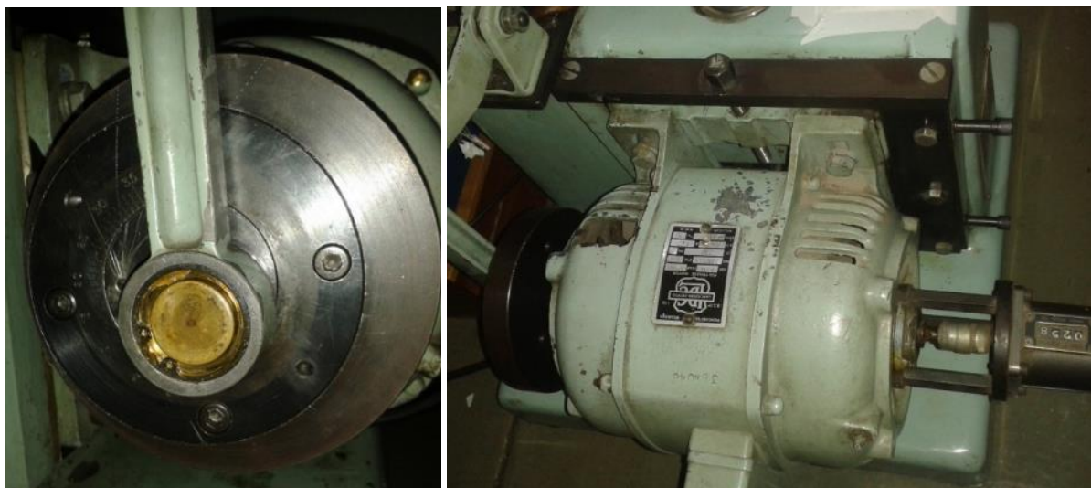
Figure 5.39 - Double Eccentric and Motor Height Adjustment Screw of the Fatigue Testing Machine
