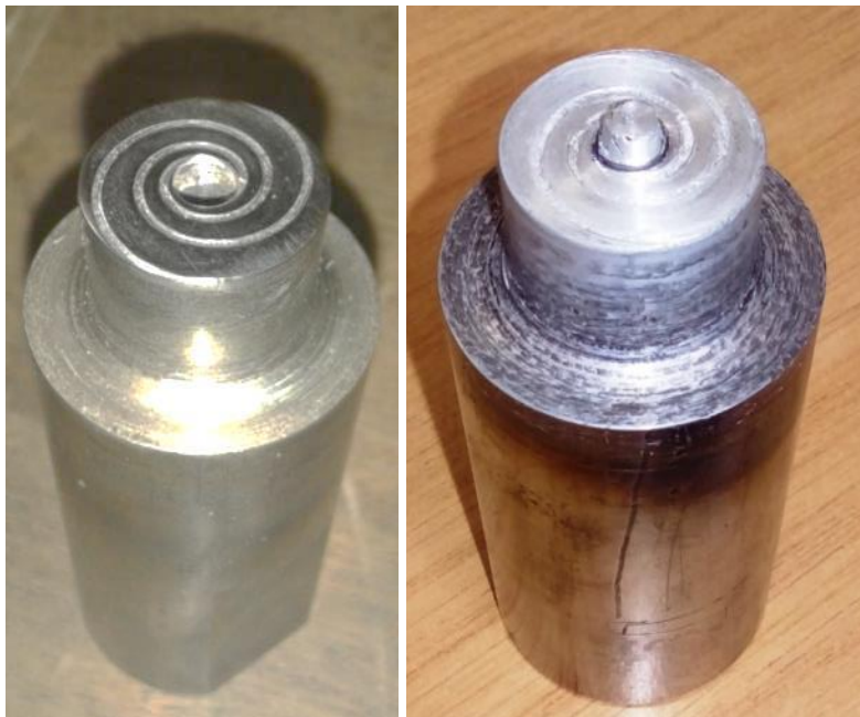
Figure 5.11 - Facetted Pin and Reduced Diameter Spiralled Shoulder Combination Friction Stir Welding Tool
