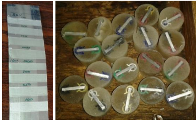
Figure 6.71 - Laser Shock Peened Strips of Varying Parameters on 1000 RPM and 400 mm/min
