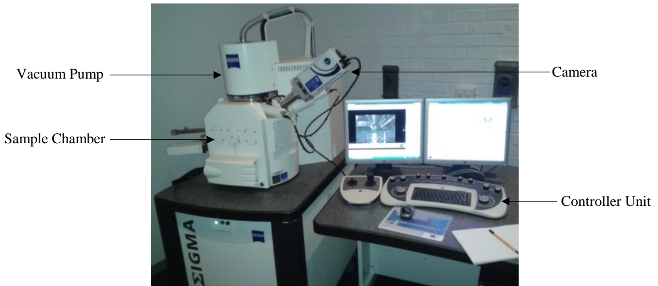
Figure 5.28 - Zeiss LEO 1525 Field Emission Gun Scanning Electron Microscope
