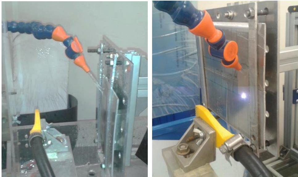
Figure 5.16 - Close View of Water Nozzle Applicator
