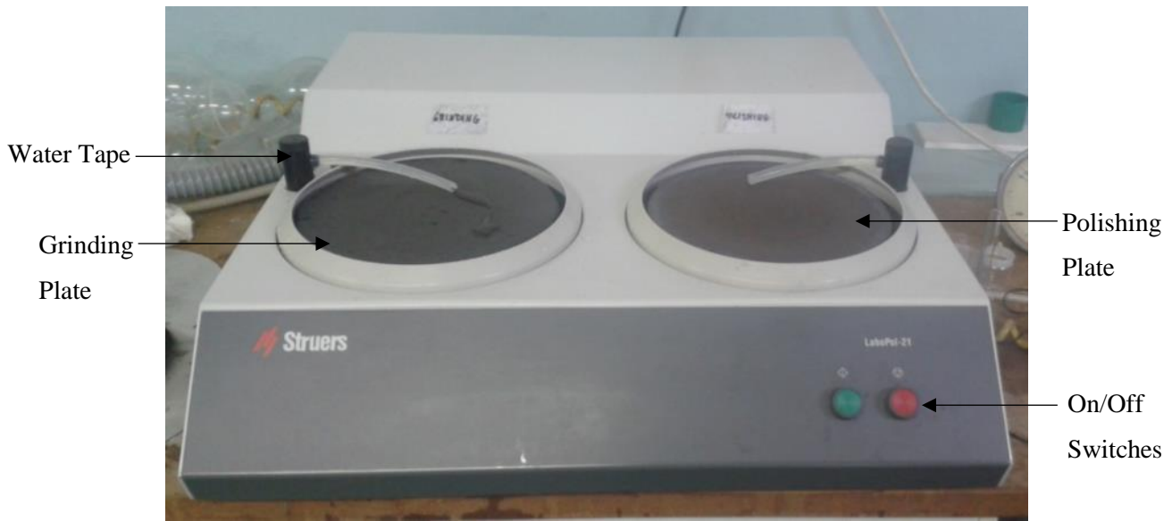
Figure 5.23 - Struers Labopol-21 Surface Grinding and Polishing Machine
