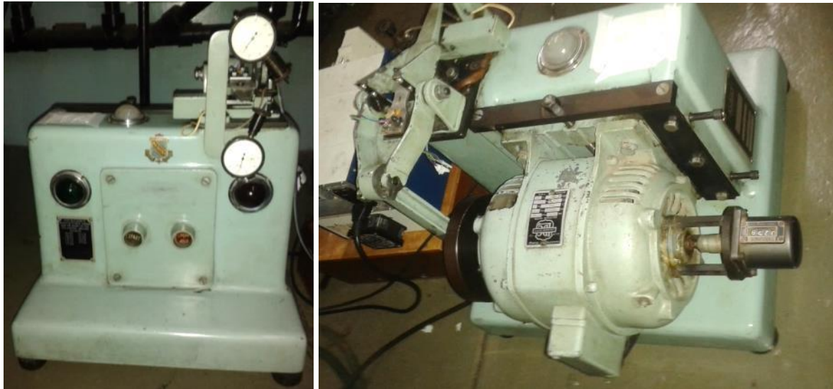
Figure 5.37 – Avery Type 7303 Bending Fatigue Apparatus
