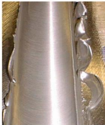
Figure 2.37 - Example of Excessive Ribbon Flash Formation during Friction Stir Welding
