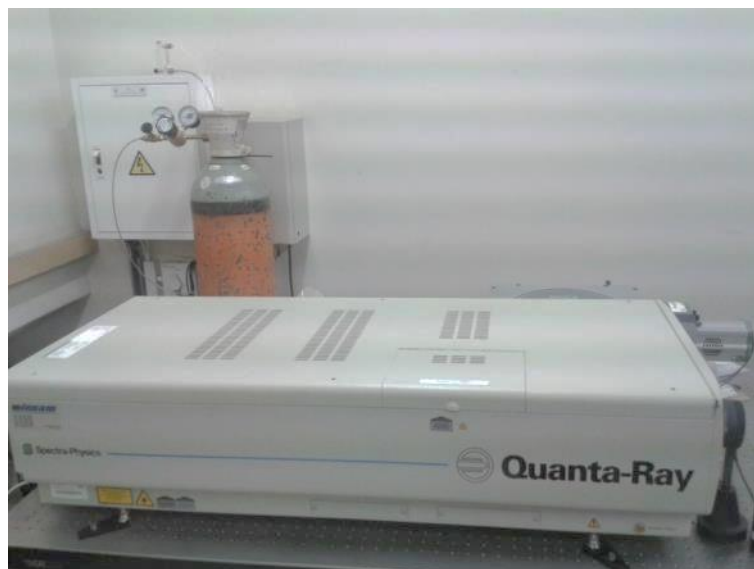
Figure 5.12 – Quanta Ray Pro- 270 Nd:Yag Laser
