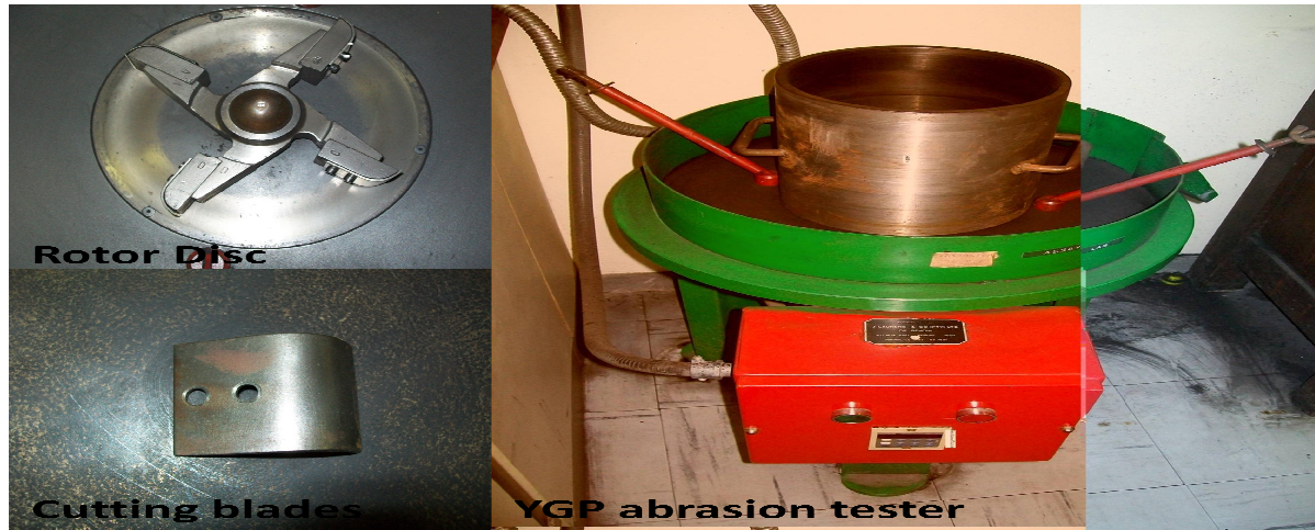
Figure 8: Abrasive index tester pot
