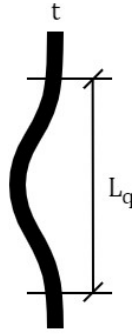
Figure 6: Elephant foot buckling half wavelength, L_q
