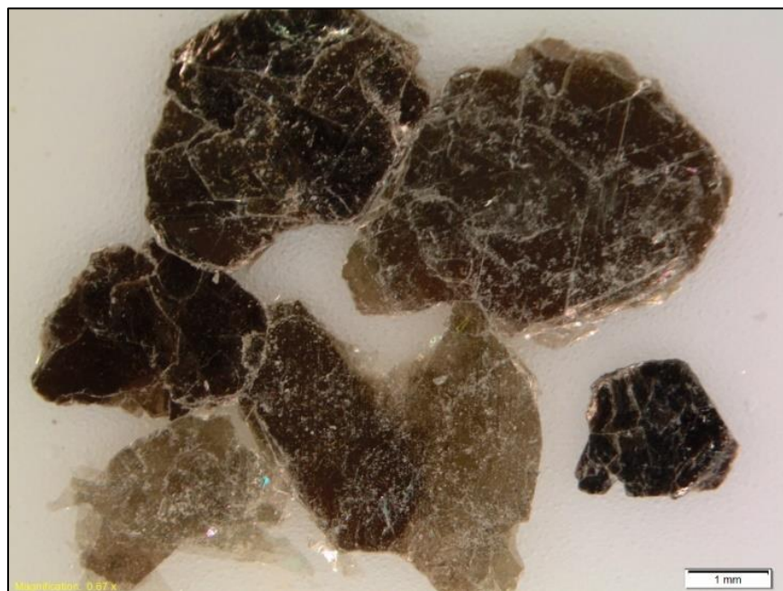
Figure 37: Phlogopite mica from 2016 RC hole 16, collected at a depth of 149m in contact between fresh carbonatite and phonolite in the centre of the Karingarab Carbonatite.
