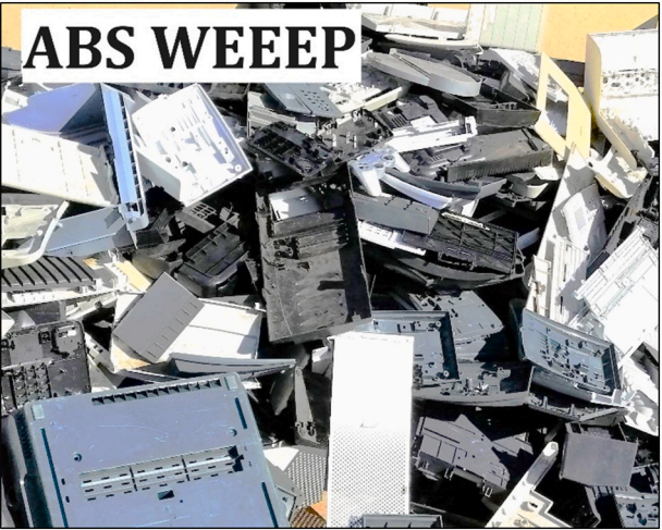
Fig. 6. Sorted and cleaned ABS WEEEP fractions.
