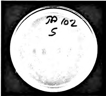
Figure 16m Positive R-factor test (Ampicillin) TA 102.
