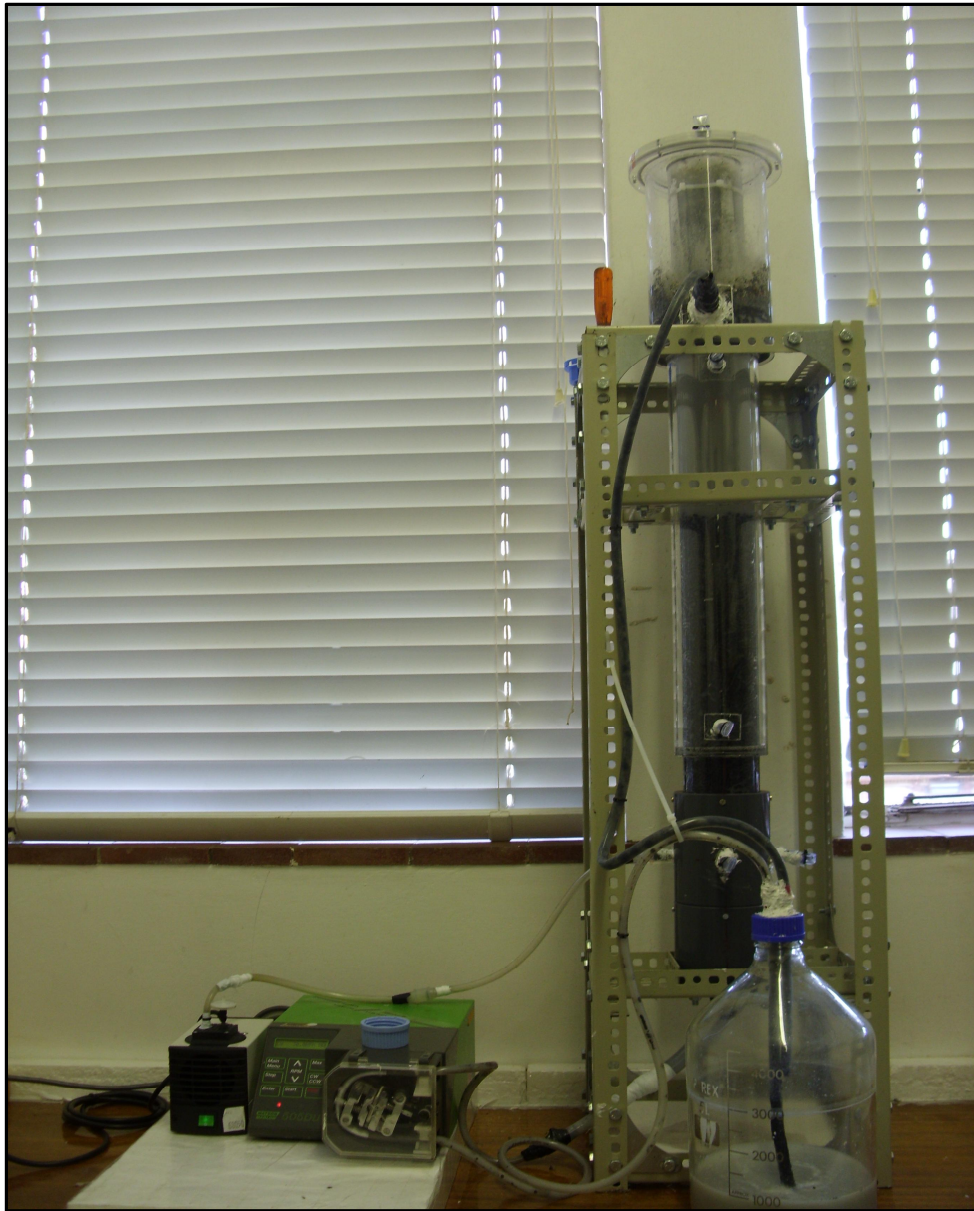
Figure 3.1b: Visual set-up of FBBR
