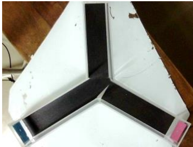
Figure 2.3: Y-Maze test apparatus consisting of three transparent Perspex arms (L – 29cm, W- 8.5cm, H – 15cm) joined at 120° & attached to a Perspex base, lined with plywood painted black to contrast the white rats.
