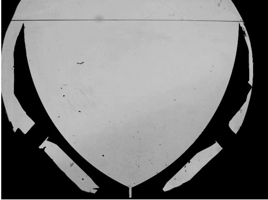
Figure 5.6: Image of an Incident Shock Entering the Test Section.
