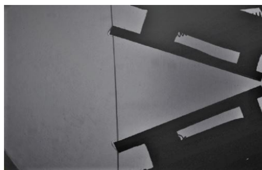
(b) Shock Coming Into Contact With Leading Edges.
