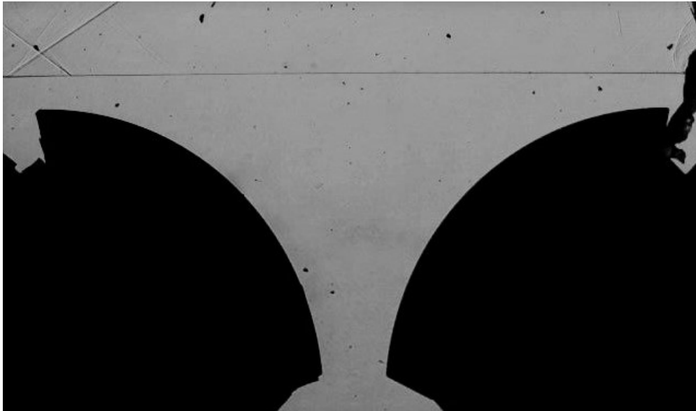
Figure 7.8: Image of Incident Wave at Mach 1.38 Entering the Test Rig in an Aligned Position.
