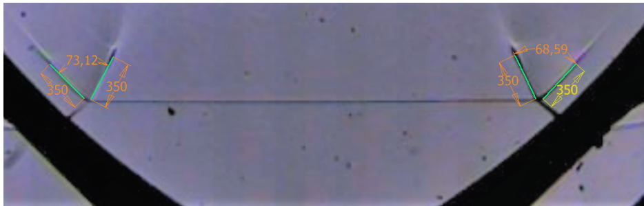
Figure 7.6: Measurement of the Angle Between the Shear Layer and Reflected Wave at Mach 1.47.
