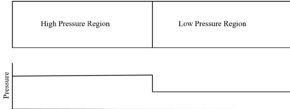
Figure 2.14: Pressure Diagram of the Shock Tube Before the Rupture of the Diaphragm
