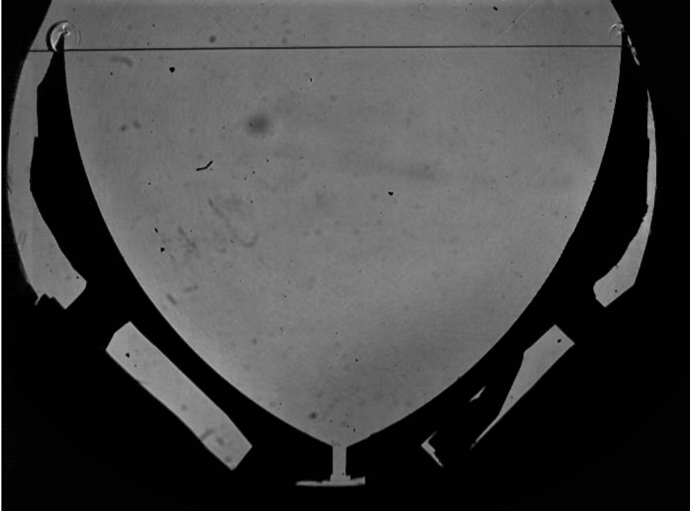
Figure 5.1: A Shock Entering the Test Rig with Concave Test Pieces Attached.
