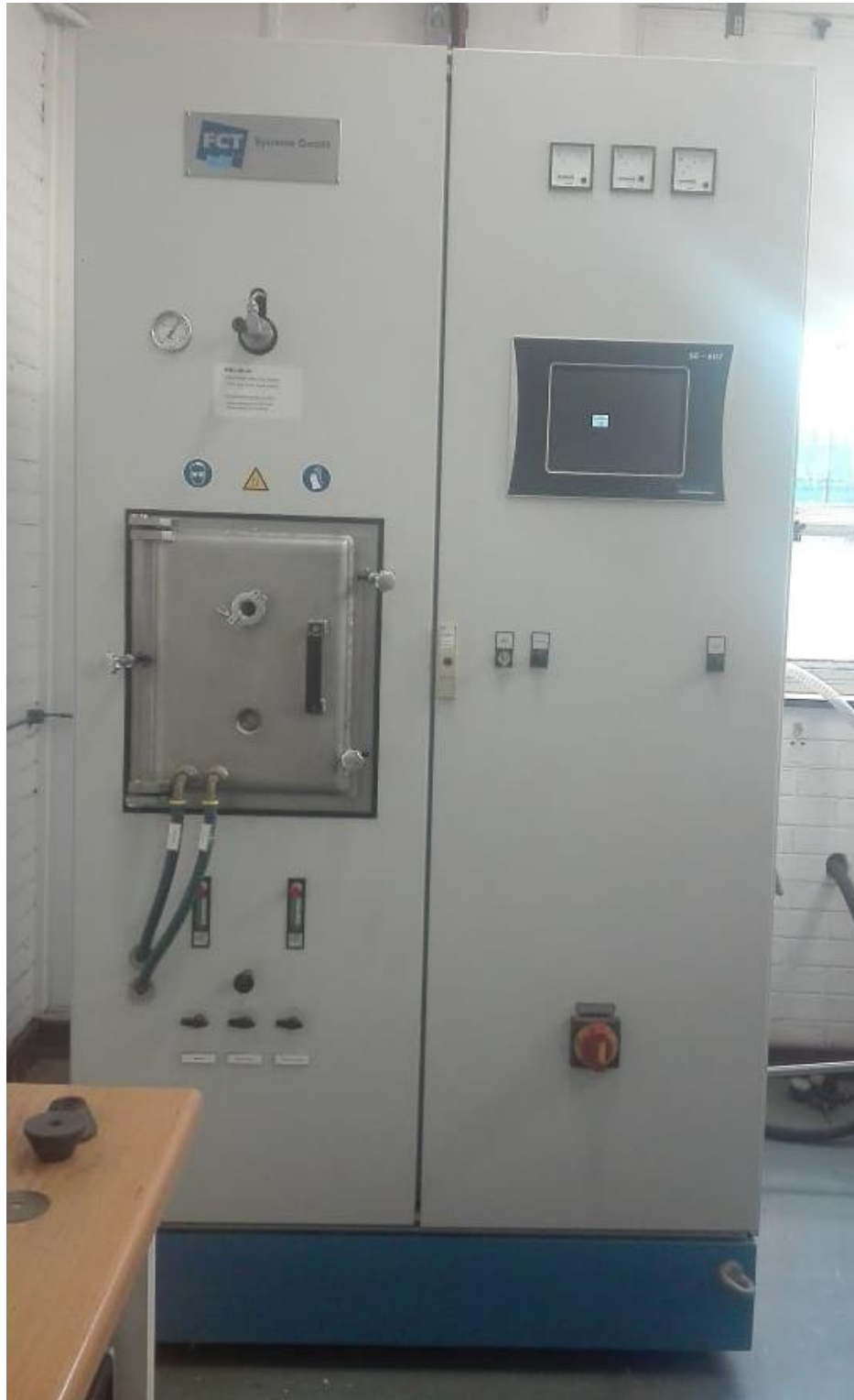
Figure 3.1: The SPS furnace used to sinter cBN-MAX powders to synthesise the composite material.
