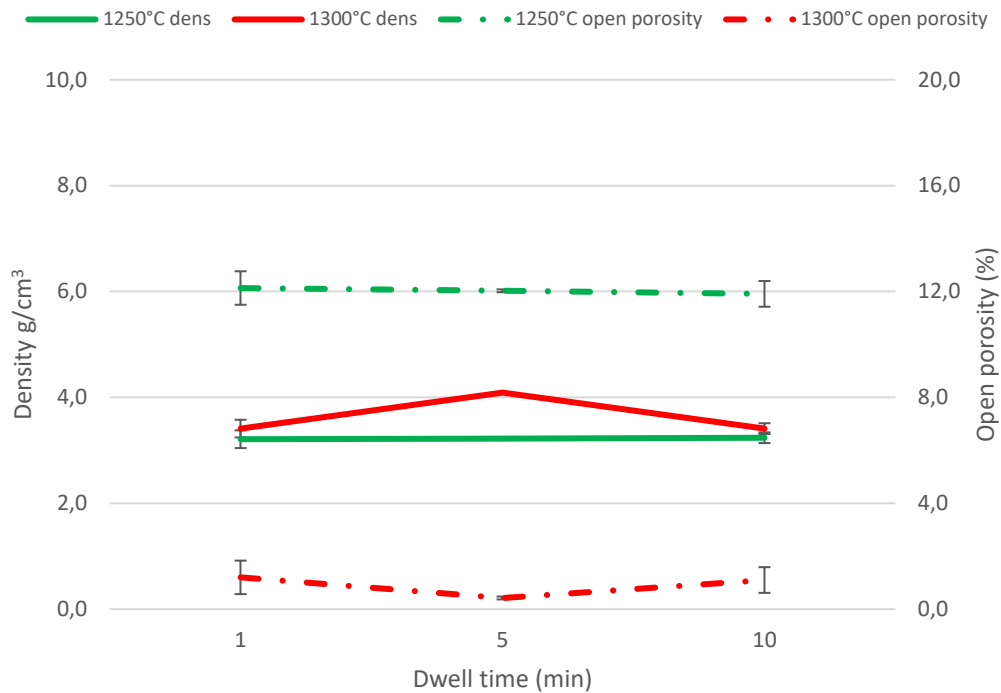
Figure 4.30: Densities and open porosities of Ti 3 AlC 2 -cBN (20 vol.%, 10 µm) samples sintered at different temperatures and for different dwell time.
