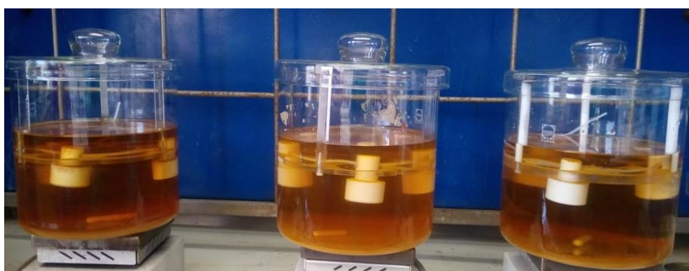
Figure 54: Fe precipitation after day 5 in the laboratory set up
