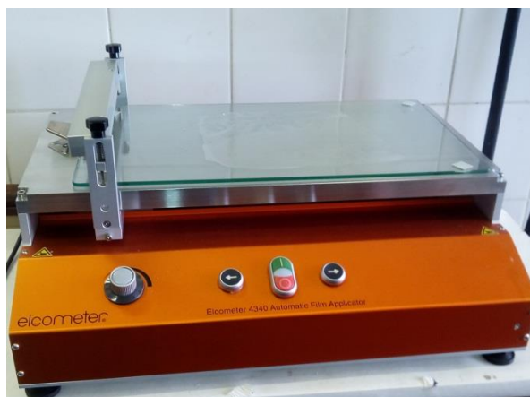
Figure 27: Elcometer motorised film applicator with casted membrane
