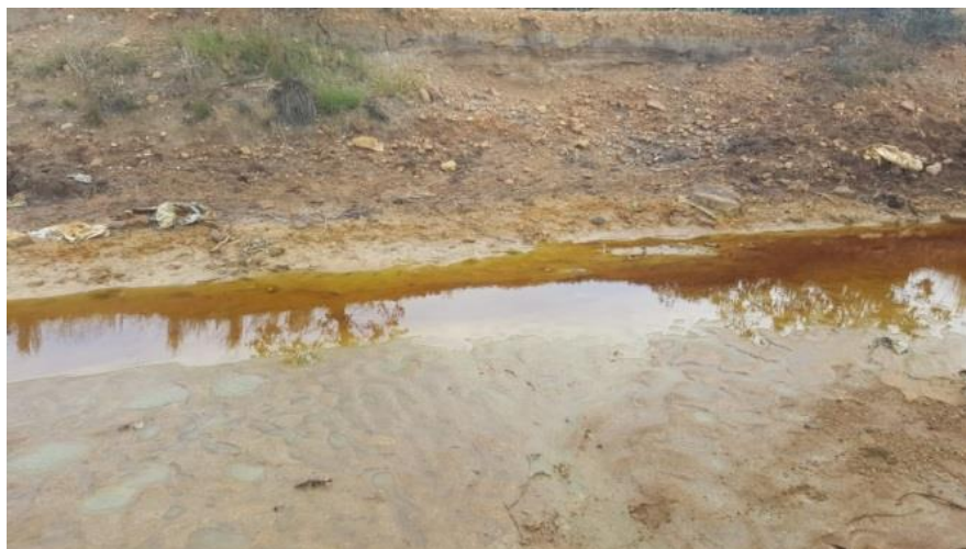
Figure 1: Acid mine drainage through a stream in Roodepoort, Johannesburg West. The sampling site was near a mine tailing, with active AMD production
