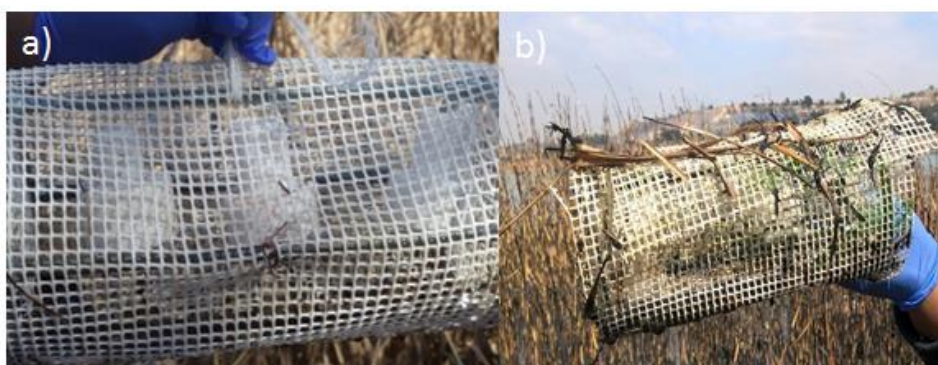
Figure 64: Picture of PIM-based passive sampler cages a) on day of deployment and b) day 12 at Fleurhof dam
