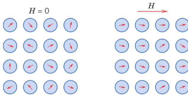
Figure 29: Schematic diagram of showing atomic dipole structure with/without an external magnetic field for a paramagnetic material [51].
