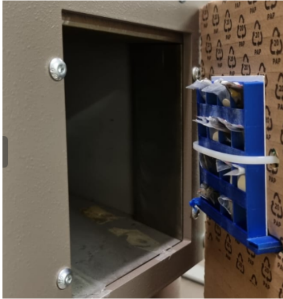
Figure 4.7: Window of the Cobalt-60 source (approximately 20 cm away from the source), along with the samples designated to receive 100 kGy, housed in one of the sample holders.
