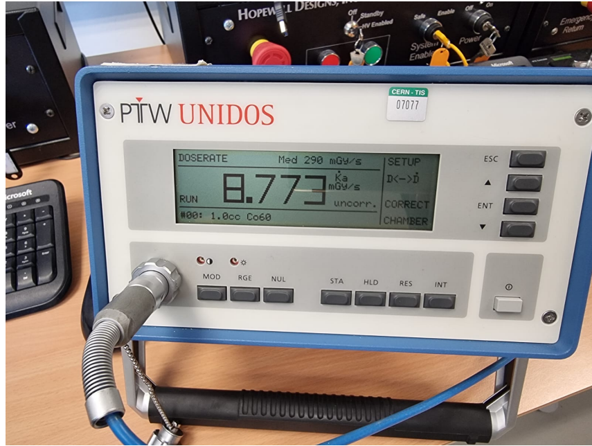
Figure 4.8: The dose reading was taken by a probe located approximately 88 cm away from the Cobalt-60 source. This is the region where the samples designated to receive 5 kGy were housed in the sample holder.
