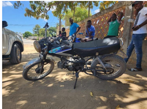
Figure 6 - Illustration of a motorcycle with a front light, but without a rear or turning light.
