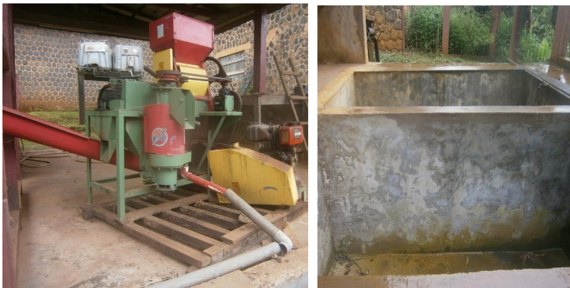
Figure 8-8: Penagos machine for fully-washed coffee and the central processing unit in the Belo ACU.
