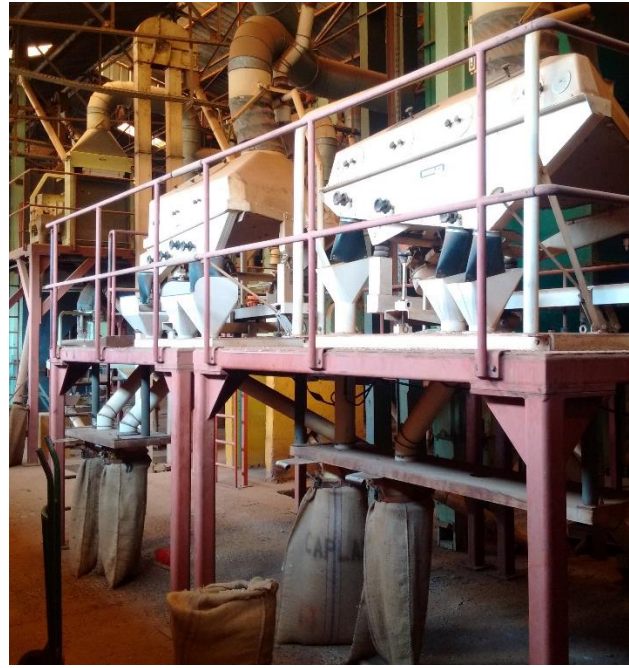
Above left: An old Tarar sorting machine does initial sorting to pick out stones and other foreign matter before coffee beans are introduced into the digital line. Top right: digital calibrator.
