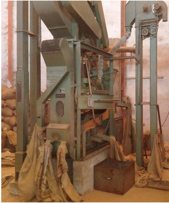
Above left: An old Tarar sorting machine does initial sorting to pick out stones and other foreign matter before coffee beans are introduced into the digital line. Top right: digital calibrator.
