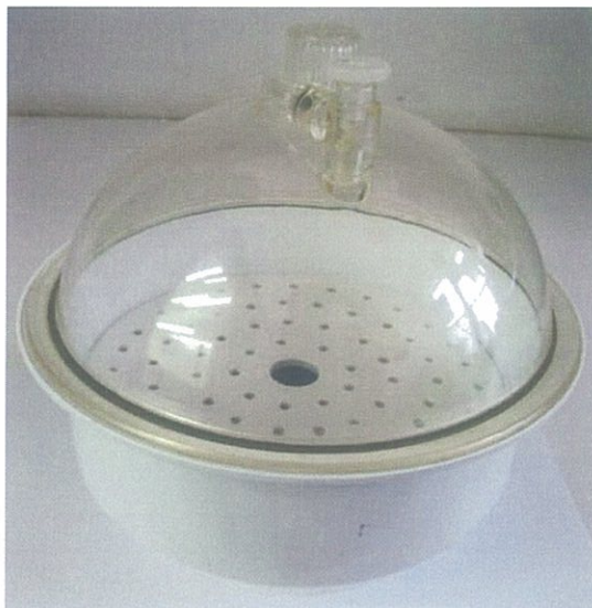
Figure 2.4: Desiccator containing activated silica gel (4.5L (v/v) with \pm 500 g silica gel)
