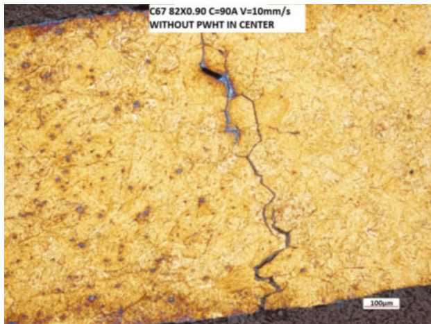
Fig. 16 The presence of a crack within the melted zone area where welding was conducted without using post-weld heat treatment [165]
