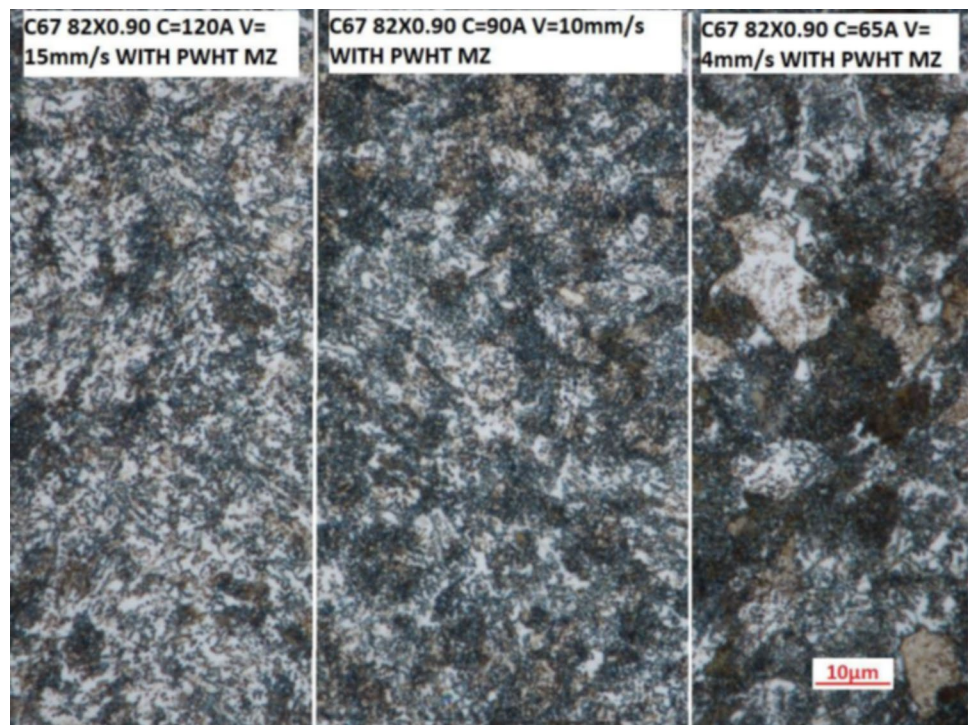
Fig. 14 The melting zone region under various welding parameters with the inclusion of post-weld heat treatment [165]
