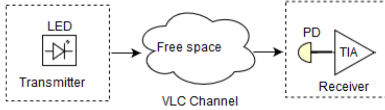
FIGURE 2.1: Typical VLC system.
