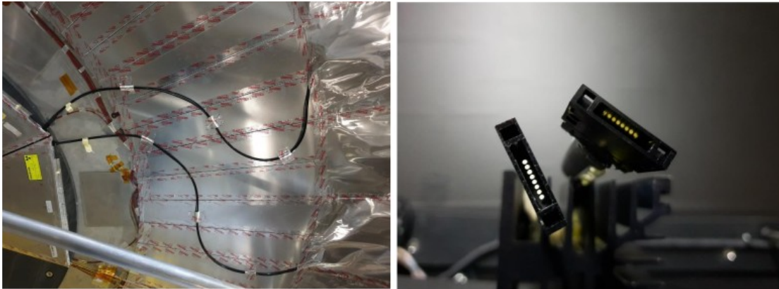
Figure A.10: A photograph of clear optical cable connecting MBTS counters to the calorimeter.
