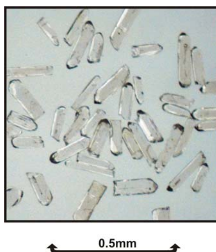
Figure 4.9 Selection of zircons from NM04-9 (migmatized granite gneiss, Sørøya). The zircons are dominated by the \{100\} prism and \{101\} pyramidal terminations. Cores are only observed in crystals with a length: width ratio \leq 1:3 . Besides this, the zircons are generally uniform in morphology and colour.
