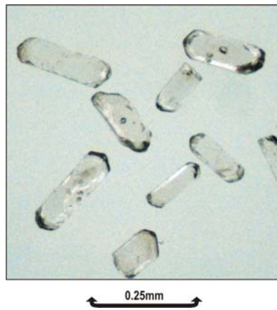
Figure 4.15 Selection of zircons from sample Co4-2 (granitic leucosome, Magerøya). The zircons have a simple prismatic morphology dominated by \{100\} prismatic and \{101\} pyramidal faces. In general the crystals are homogeneous in colour and fluid inclusions are commonly observed.
