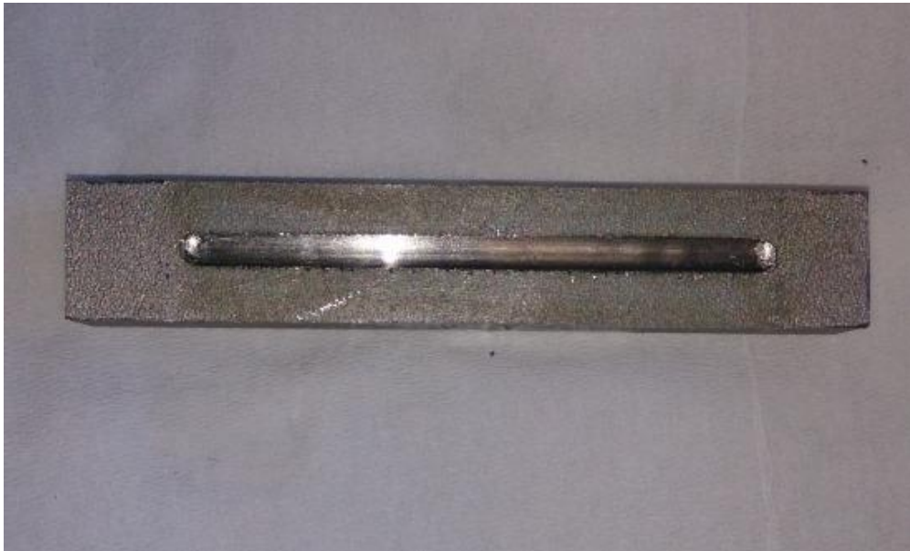
Figure 4. 25: Typical wear track on the steel counterfaces caused by the WC-6 wt.% Co buttons during sliding.
