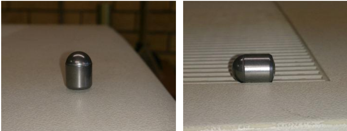
Figure 3. 1: Physical appearance of the cemented carbide buttons.
