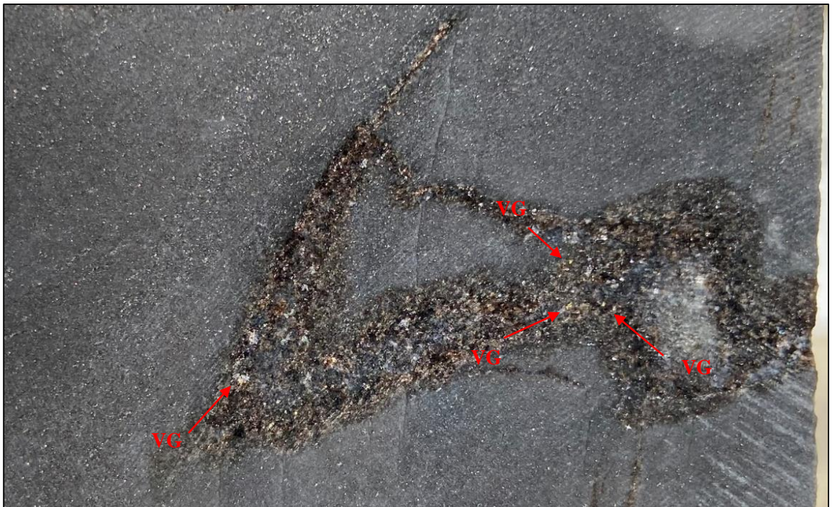
Figure 41 . Quartz veinlets with biotite selvages contain pyrrhotite, arsenopyrite, and visible gold (VG) grains. The bottom left arrow shows a VG grain surrounded by arsenopyrite crystals. The host rock is light grey (bleached), fine-grained metagreywacke with fine-grained acicular arsenopyrite disseminated within the groundmass OKD274@ 201.34m, The Bulge section of the Twin Hills Gold Deposit).
