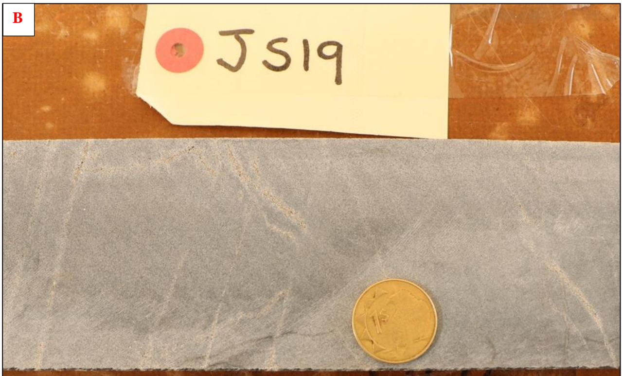
Figure 15 Photographs of borehole core showing A) Interbedded metagreywacke (IMGK) in a pelitic zone with graded bedding characterized by pale, quartz-rich bases, and dark grey, mica-rich tops. B) Massive metagreywacke (MGWK) with distinctive low to moderate schistosity and significantly higher quartz abundance and minor micaceous minerals.
