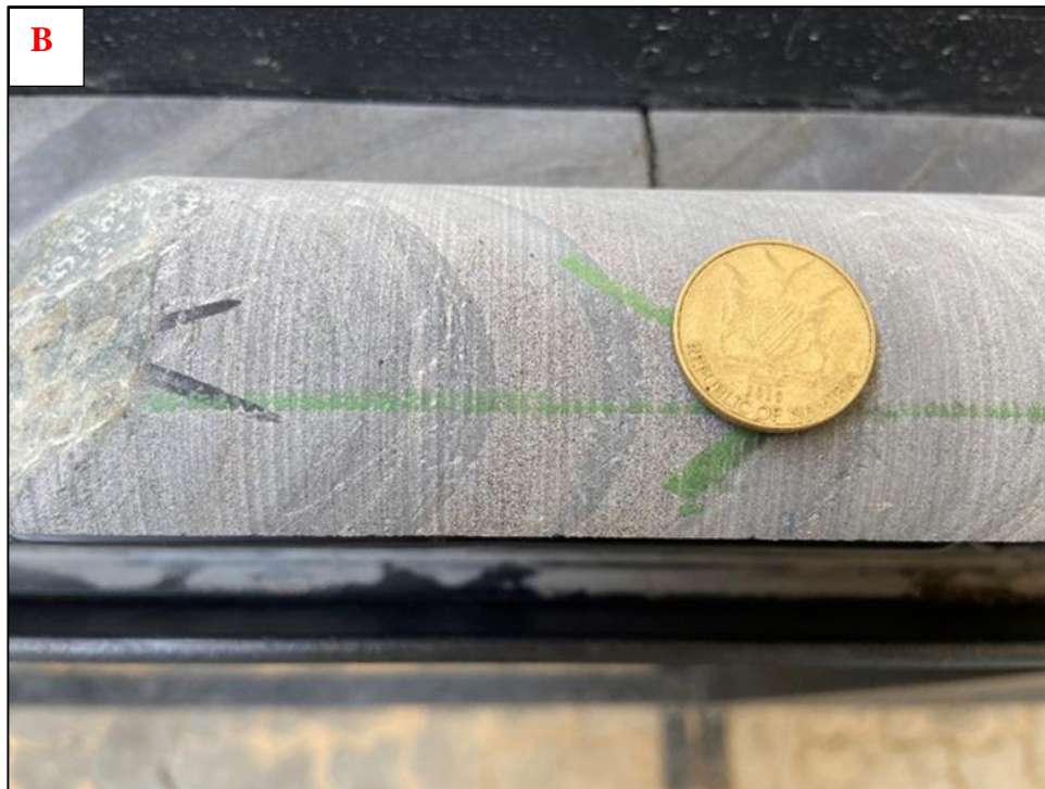
Figure 12 Photographs of borehole core showing A) Interbedded metagreywacke in a pelitic zone. B) Interbedded metagreywacke in a psammitic zone with coarser beds, graded bedding characterized by coarser, quartz-rich bases, and finer mica-rich tops.
