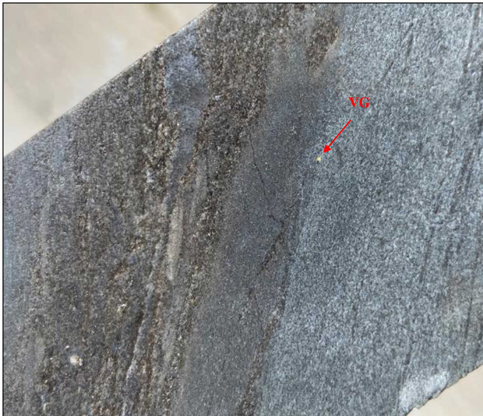
Figure 36 Light grey (bleached) fine-grained interbedded metagreywacke, silicified and potassic alteration mainly characterized by quartz veinlets with biotite selvages. VG within the groundmass. OKD189 @ 186.92m, Clouds East section of the Twin Hills Gold Deposit.
