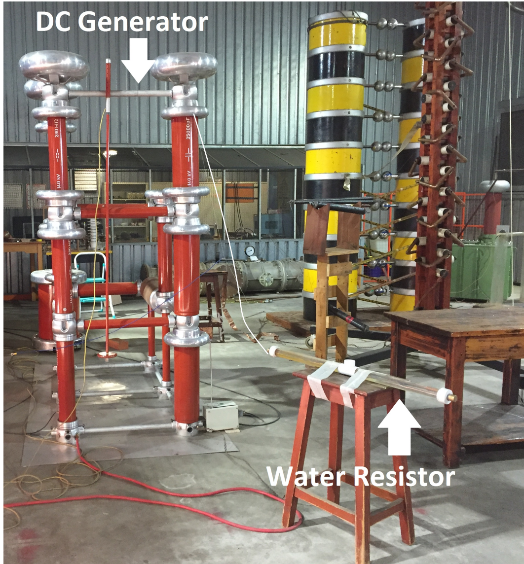
FIGURE 4.8: Image of the laboratory DC generator connection to water resistor that connects to the HV rod.
