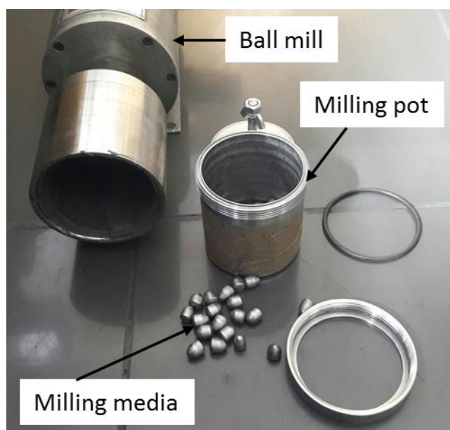
Figure 3.1: Laboratory scale ball mill.
